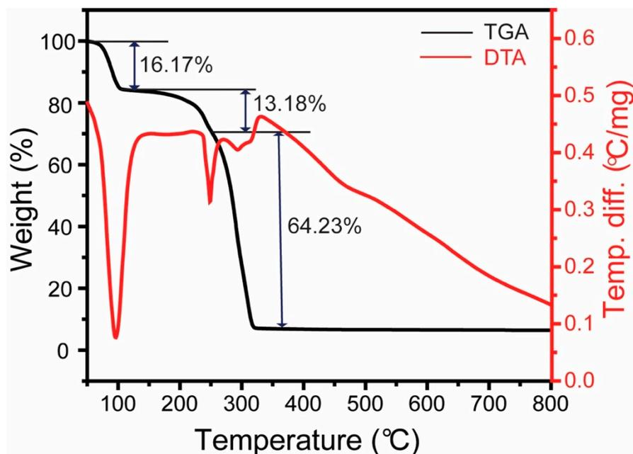
Figure 5. Thermogravimetry/differential thermal analysis (TG/DTA) of the ZAD.
