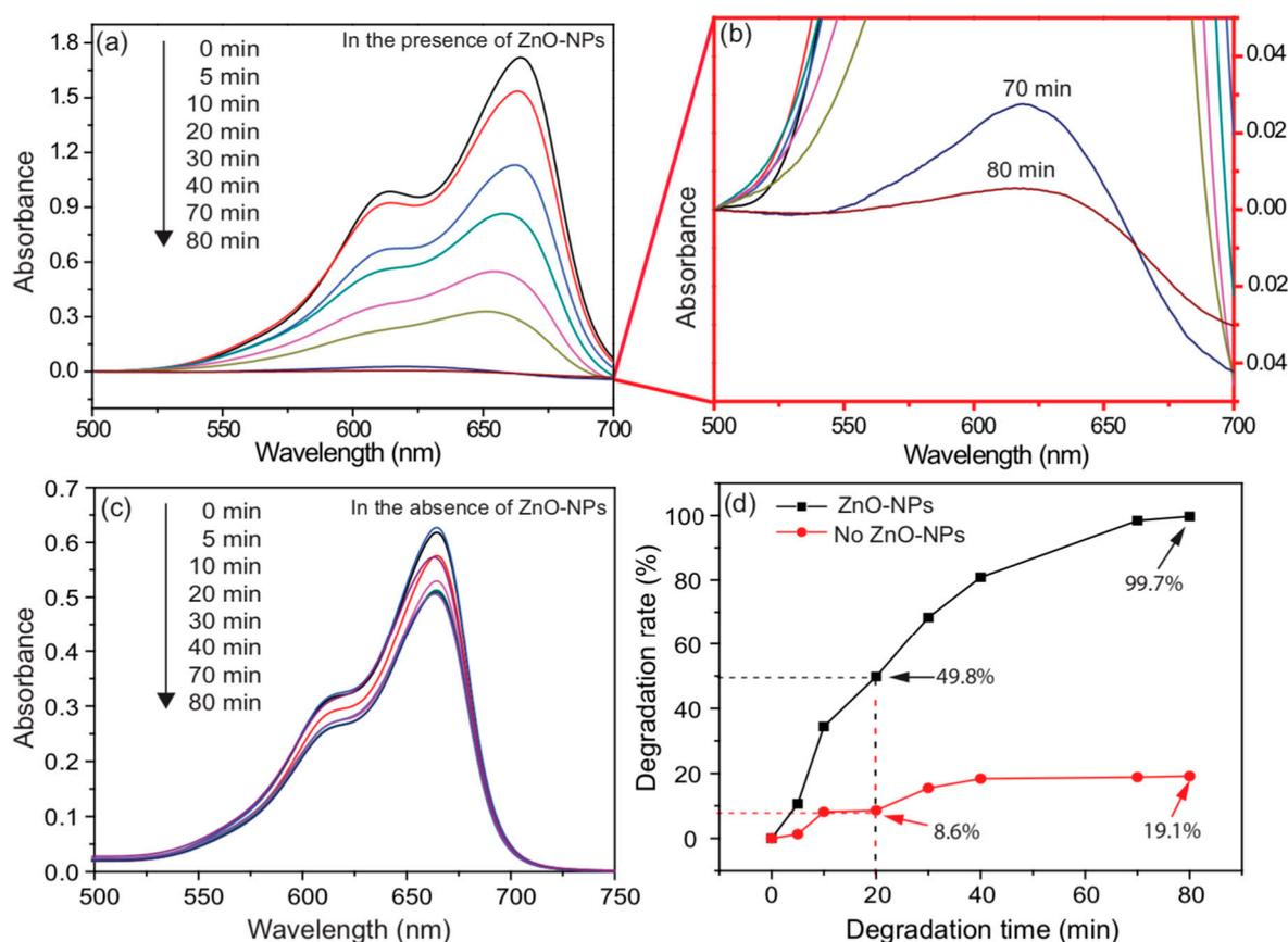
**Figure 6.** (a) UV-vis absorbance spectra showing the decomposition of methylene blue (MB) in the presence of ZnO-NPs, (b) a magnified view of the curves in panel (a), (c) UV-vis absorbance spectra of MB decomposition in the absence of ZnO-NPs, (d) degradation rates of MB in the presence or in the absence of ZnO-NPs. The decomposition of MB was carried out at 29 °C.
