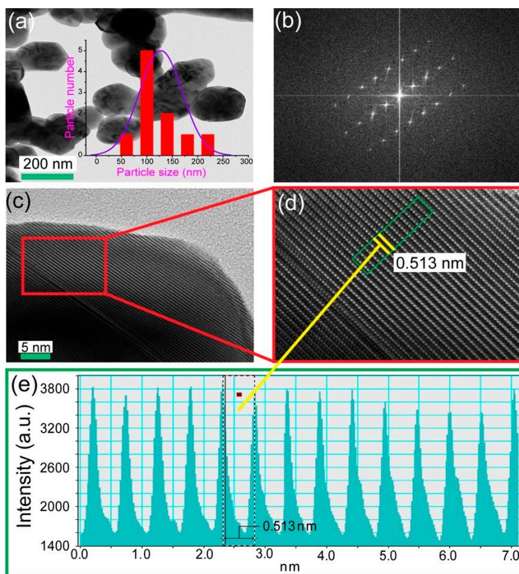
**Figure 3.** (a) Typical transmission electron microscopy (TEM) image of synthesized ZnO-NPs; the inset shows the corresponding particle size distribution of the ZnO-NPs. (b) The selected-area electron diffraction (SAED) pattern, (c) high-resolution TEM image, (d) inverse fast Fourier transform (IFFT) spectrum, and (e) profile of the IFFT image in (d).
