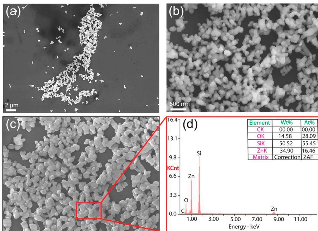
**Figure 2.** (a) and (b) field-emission scanning electron microscopy (FE-SEM) images of the prepared ZnO-NPs at different magnifications; (c) FE-SEM image showing the region selected for EDS analysis and (d) the corresponding EDS spectrum of the ZnO-NPs.
