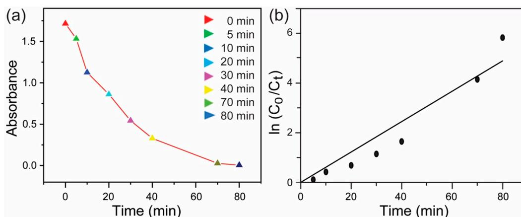
**Figure 7.** Photocatalytic performance of the ZnO-NPs: (a) absorbance vs time and (b) kinetic study for MB degradation (linear fitting data).
