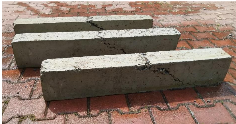
Figure 20. Reinforced concrete (RC) Beams with shear crack.
