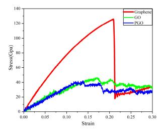
Figure 4. The stress-strain curves under uniaxial tension.
