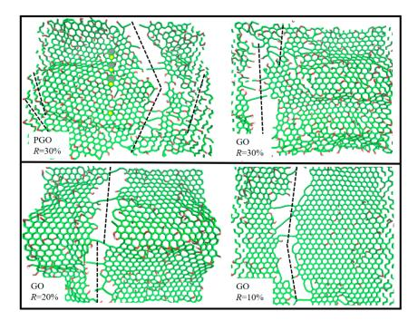
Figure 6. Tensile failure process of polycrystalline graphene oxide and graphene oxide at different R.
