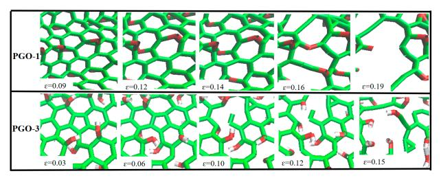
Figure 10. Fracture and reconstruction of the bonds between PGO-1 and PGO-3.
