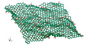
Figure 2. Model of polycrystalline graphene oxide after relaxation.
