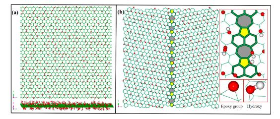
**Figure 1.** (a) Graphene oxide (GO) model; (b) polycrystalline graphene oxide (PGO) model (carbon atoms and carbon–carbon bonds are shown in green, oxygen atoms in red, and hydrogen atoms in white).
