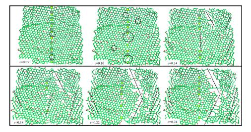
Figure 5. Tensile failure process of polycrystalline graphene oxide.
