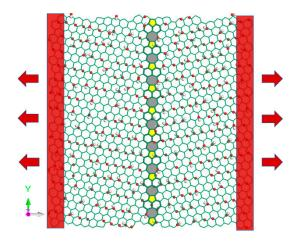
Figure 3. Tensile diagram of polycrystalline graphene oxide.
