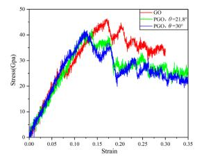
**Figure 7.** Uniaxial tensile stress-strain curves at R = 30%.
