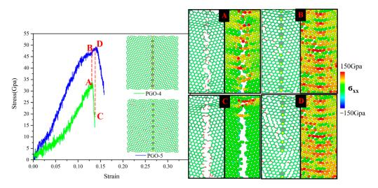
**Figure 11.** Uniaxial tensile stress-strain diagram and model diagram of pgo-4 and pgo-5 (**left frame**), bond fracture diagram and atomic stress distribution diagram of corresponding marked points (**right frame**). Points A and B: The moment when PGO-4 reaches the ultimate stress; Points C and D: The moment when PGO-5 reaches the ultimate stress.
