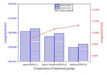
Figure 9. Energy change of PGO during the tensile process.
