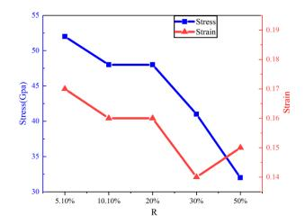
**Figure 8.** Ultimate stress and ultimate strain values of PGO under different oxygen content ( $\theta = 21.8^{\circ}$ ).
