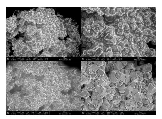
**Figure 8.** SEM results for a sample containing ammonium nitrate and calcium carbonate (P2) at room temperature (**a**,**b**) and at 130–180 °C (**c**,**d**).
