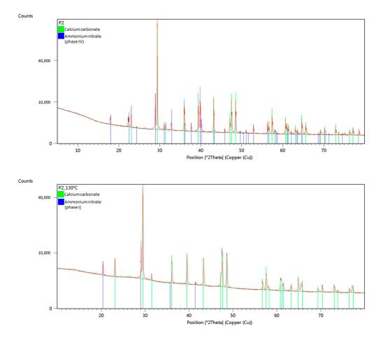
Figure 7. XRD results for a sample containing ammonium nitrate and calcium carbonate (P2) at room temperature and at 130 °C.
