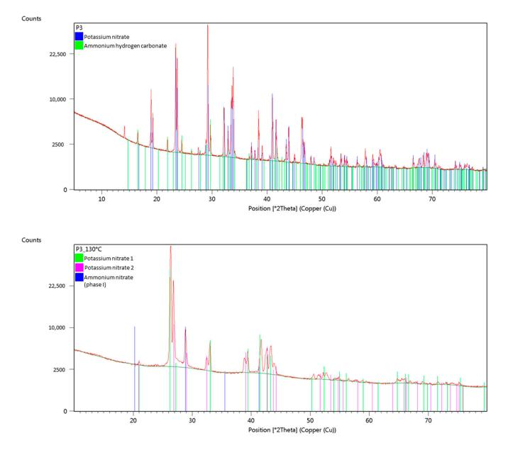
**Figure 11.** XRD results for a sample containing ammonium nitrate and potassium hydrogen carbonate (P3) at room temperature and at 130 °C.
