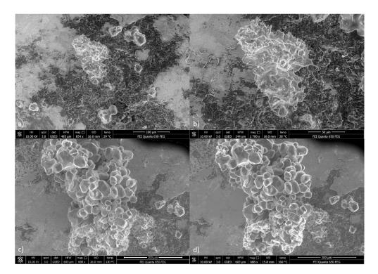
**Figure 16.** SEM results for a sample containing ammonium nitrate and potassium carbonate (P4) at room temperature (**a**,**b**) and at 130–160  $^{\circ}$ C (**c**,**d**).
