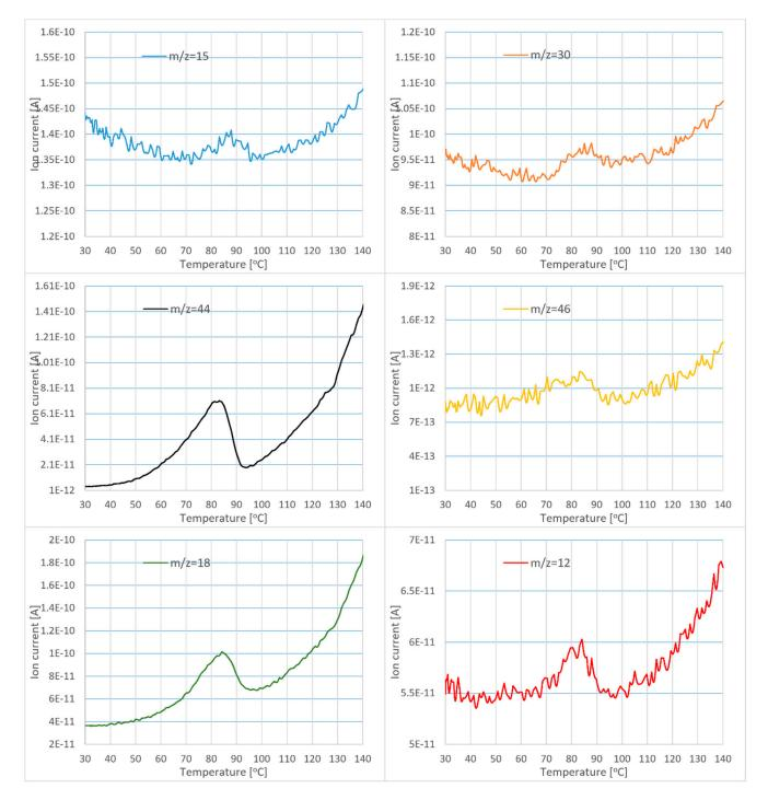
Figure 10. MS results for a sample containing ammonium nitrate and potassium hydrogen carbonate (P3).
