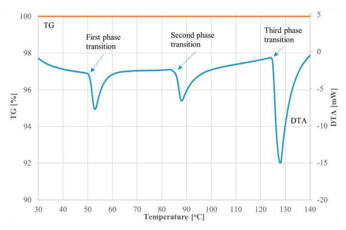
Figure 1. DTA-TG results for a pure ammonium nitrate sample (P1).
