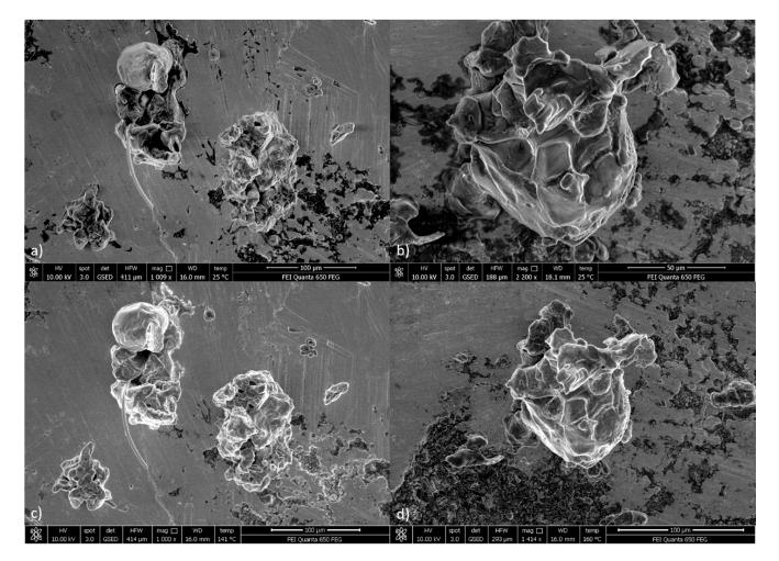
**Figure 12.** SEM results for a sample containing ammonium nitrate and potassium hydrogen carbonate (P3) at room temperature (a,b) and at 141–160 °C (c,d).
