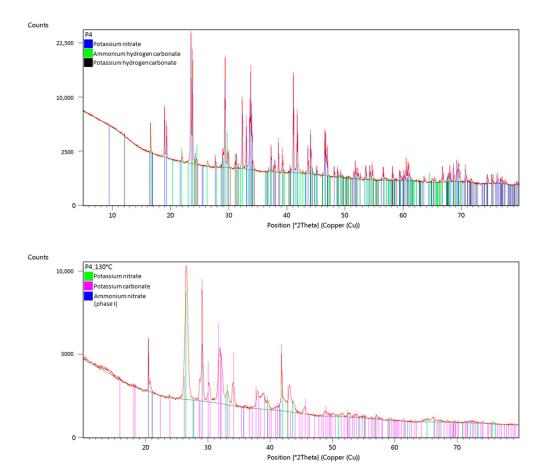
Figure 15. XRD results for a sample containing ammonium nitrate and potassium carbonate (P4) at room temperature and at 130 °C.
