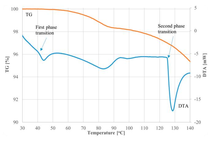
Figure 9. DTA-TG results for a sample containing ammonium nitrate and potassium hydrogen carbonate (P3).
