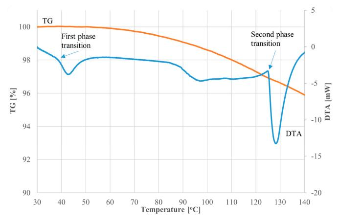
Figure 13. DTA-TG results for a sample containing ammonium nitrate and potassium carbonate (P4).
