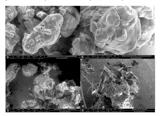
Figure 4. SEM results for a pure ammonium nitrate sample (P1) at room temperature (**a**,**b**) and at 130 °C (**c**,**d**).
