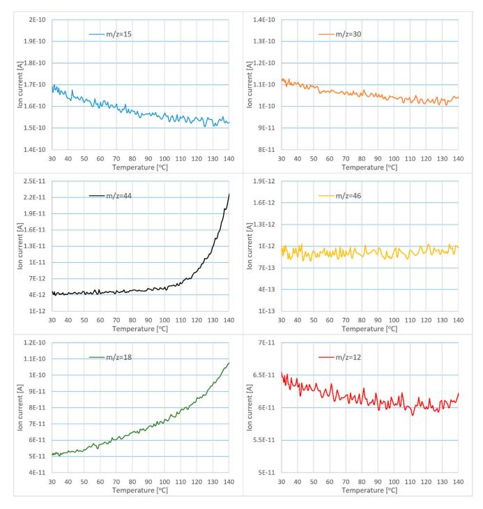
Figure 6. MS results for a sample containing ammonium nitrate and calcium carbonate (P2).
