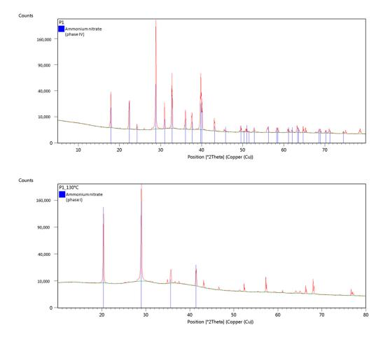
Figure 3. XRD results for a pure ammonium nitrate sample (P1) at room temperature and at 130 °C.
