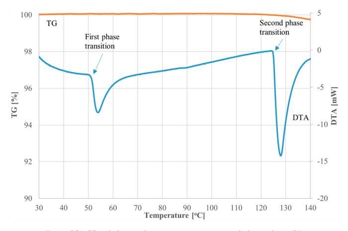
Figure 5. DTA-TG results for a sample containing ammonium nitrate and calcium carbonate (P2).
