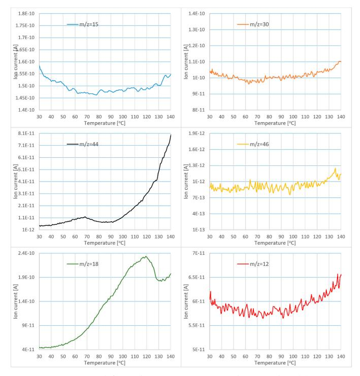
Figure 14. MS results for a sample containing ammonium nitrate and potassium carbonate (P4).
