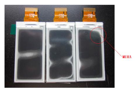
Figure 4. There is mura after 15 days of HTHH testing.
