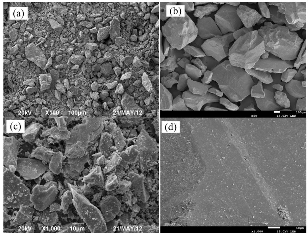
**Figure 1.** Microstructure of fluorine-bearing iron concentrate (a,c) and specularite (b,d).
