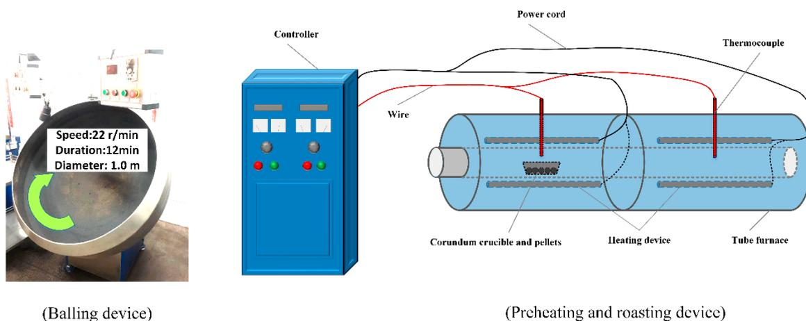
**Figure 3.** Schematic diagram of balling, preheating and roasting devices.
