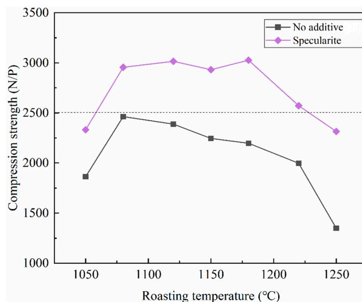
**Figure 6.** Effects of roasting temperature on compression strength of roasted pellets (preheating temperature 950 °C, preheating time 14 min, roasting time 10 min) (a horizontal dotted line at 2500 N/P is the first-grade qualified standard for blast furnace [20]).
