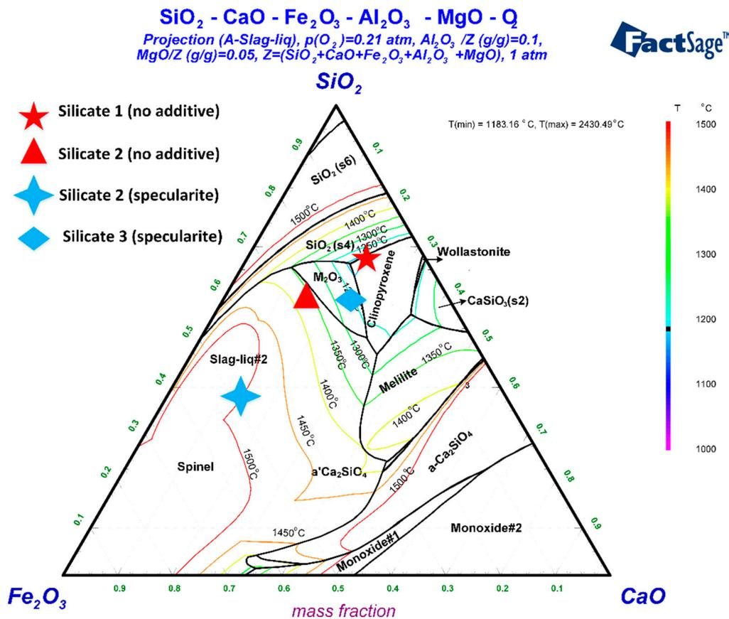
**Figure 10.** Phase diagram of SiO<sub>2</sub>-CaO-Fe<sub>2</sub>O<sub>3</sub>-10wt%Al<sub>2</sub>O<sub>3</sub>-5wt%MgO-O<sub>2</sub>(P<sub>(O<sub>2</sub>)</sub> = 0.21) calculated by FactSage 8.0 (marked locations according to Table 5).
