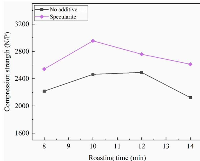
**Figure 7.** Effects of roasting time on compression strength of roasted pellets (preheating temperature 950 °C, preheating time 14 min, roasting temperature 1080 °C).
