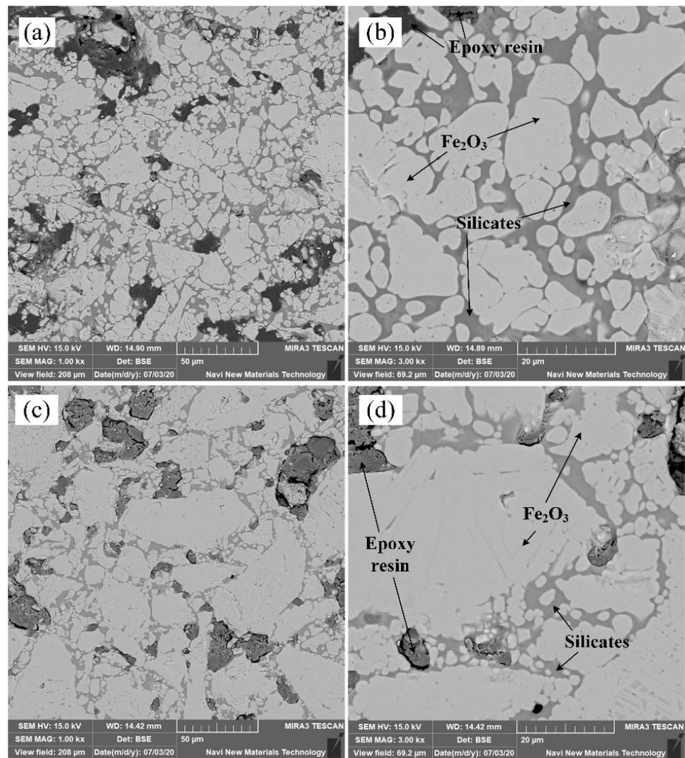
**Figure 8.** Microstructure of roasted fluorine-bearing iron concentrate pellet without (a,b) and with specularite (c,d) (preheating at 920 °C for 16 min and roasting at 1080 °C for 10 min).
