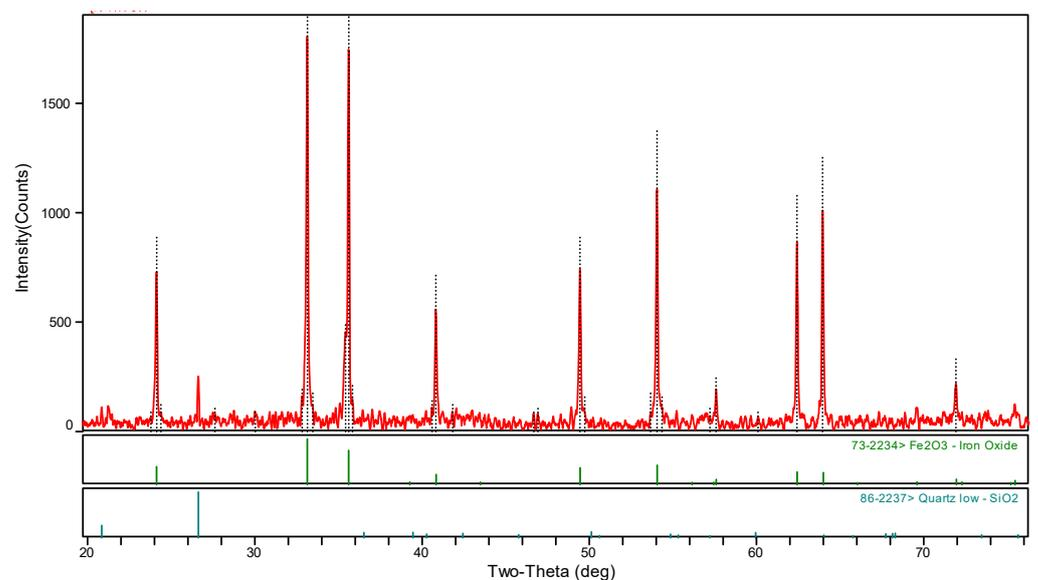
**Figure 2.** XRD patterns of the specularite.
