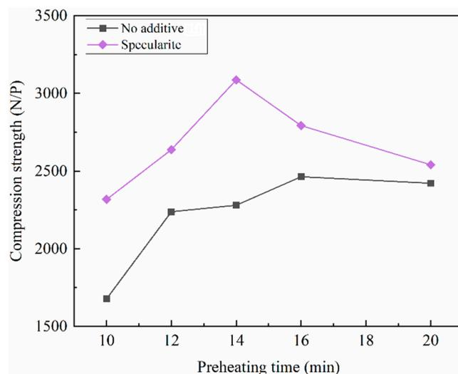
**Figure 5.** Effects of preheating time on compression strength of roasted pellets (preheating temperature 950 °C, roasting temperature 1080 °C, roasting time 10 min).
