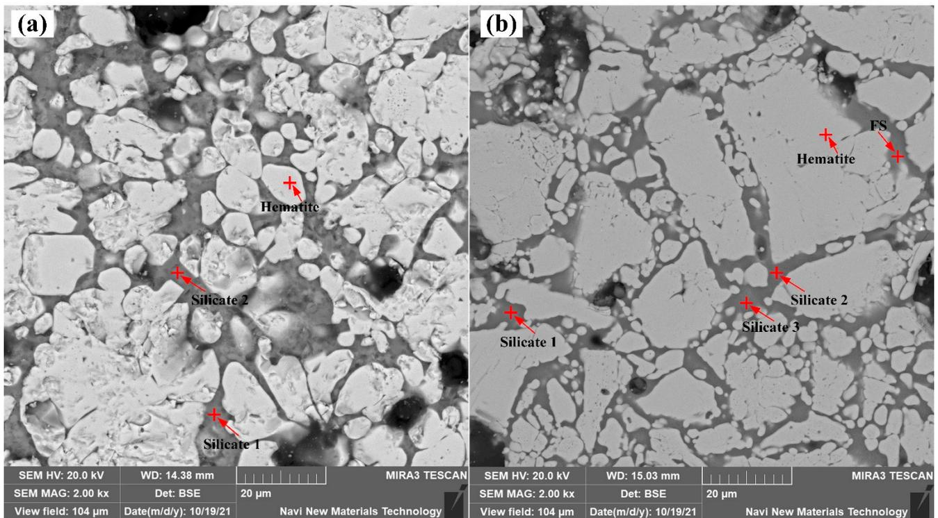
**Figure 9.** EDS analysis of roasted fluorine-bearing iron concentrate pellets with no additive (a) and adding specularite (b) (preheating at 920 °C for 16 min and roasting at 1080 °C for 10 min).
