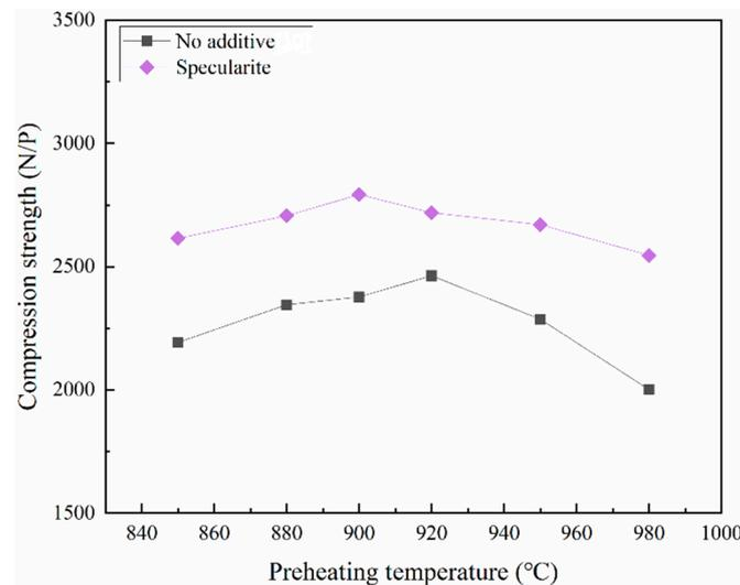
**Figure 4.** Effects of preheating temperature on compression strength of roasted pellets (preheating time 16 min, roasting temperature 1080 °C, roasting time 10 min).
