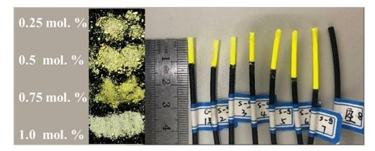
**Figure 1.** Eight YAG: Ce dosimeters with different parameters were made with the physical graph shown on the right side. On the left side are phosphors prepared via the sol-gel method; the color deepened as the concentration of Ce became higher; from top to bottom are YAG: Ce powders with Ce concentration of 0.25 mol.%, 0.5 mol.%, 0.75 mol.%, and 1 mol.%.
