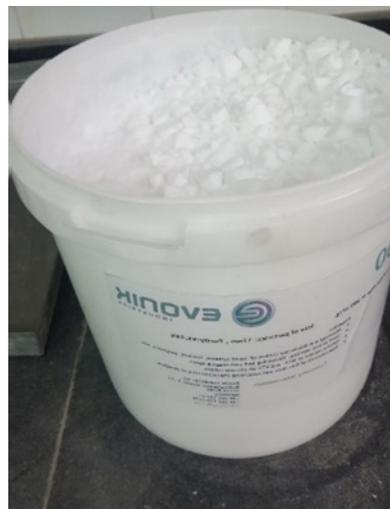
**Figure 2.** The nano-silica powder.
