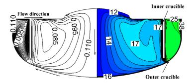
(b) Inner crucible radius of 210 mm
