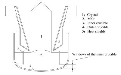
**Figure 1.** Schematic diagram of the continuous-feeding Czochralski method (CCZ) furnace with double crucibles.
