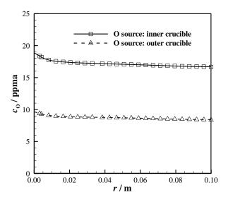
**Figure 6.** Impacts of the inner crucible and outer crucible on the oxygen distribution (ppma) at the m-c interface.
