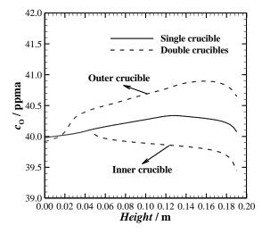
Figure 4. The oxygen distribution (ppma) at crucible walls.
