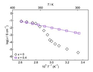
**Figure S3.** Arrhenius plots of the lithium-ion conductivities for the compounds with x = 0 (Li(CB<sub>9</sub>H<sub>10</sub>)) and x = 0.4 (0.6Li(CB<sub>9</sub>H<sub>10</sub>)–0.4Li<sub>2</sub>(B<sub>12</sub>H<sub>12</sub>)).
