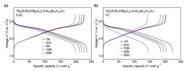
**Figure S7.** Discharge–charge profiles for the  $TiS_2/0.6Li(CB_9H_{10})-0.4Li_2(B_{12}H_{12})/Li$  cells for rates of (a) 0.2C and (b) 1C.
