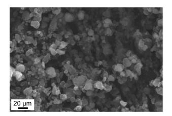
Figure S4. SEM micrograph of the x = 0.4 (0.6Li(CB<sub>9</sub>H<sub>10</sub>)–0.4Li<sub>2</sub>(B<sub>12</sub>H<sub>12</sub>)) compound.
