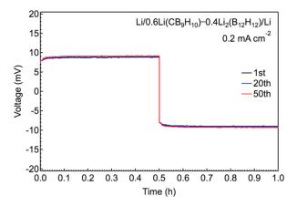
Figure S6. Galvanostatic cycling profiles of a Li/0.6Li(CB9H10)–0.4Li2(B12H12)/Li cell at 0.2 mA cm<sup>-2</sup>.
