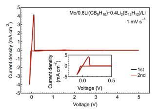
**Figure S5.** Cyclic voltammograms of a Mo/0.6Li(CB<sub>9</sub>H<sub>10</sub>)-0.4Li<sub>2</sub>(B<sub>12</sub>H<sub>12</sub>)/Li cell at a scan rate of 1 mV s<sup>-1</sup> during two cycles. Insets show the magnified plots in the low-voltage region.
