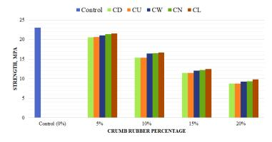
**Figure 9.** Compressive strength at 28 days.
