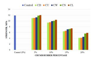
Figure 8. Compressive strength at 7 days.
