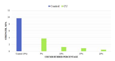
Figure 11. Compressive strength (after heating) at 28 days.
