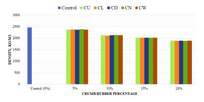
Figure 6. Density of concrete at 28 days.
