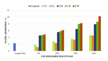
Figure 3. Water absorption at 7 days.
