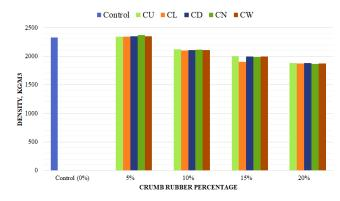
Figure 5. Density of concrete at 7 days.
