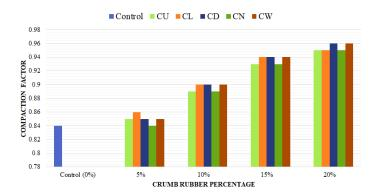
Figure 2. Compaction factor results.
