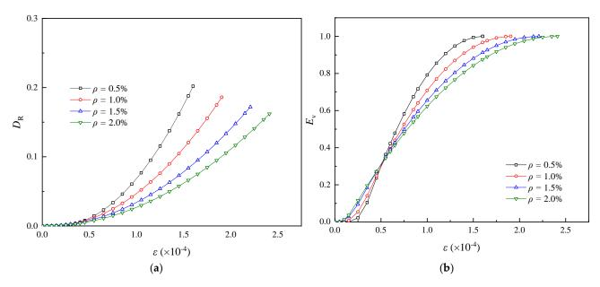
**Figure 13.** Evolution curves of damage variable and evolution factor: (a)  $D_{\rm R}$ - $\varepsilon$  curves; (b)  $E_{\rm v}$ - $\varepsilon$  curves.
