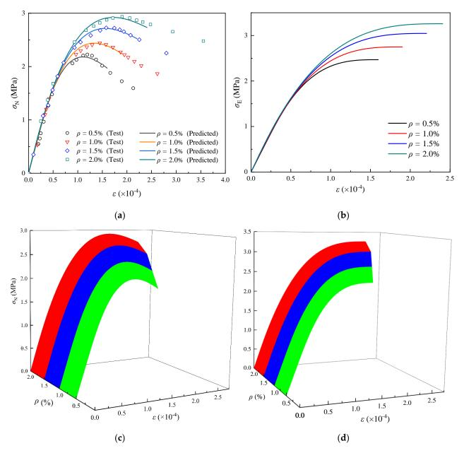
**Figure 11.** Stress–strain curves under uniaxial tension: (**a**) nominal stress–strain curve (Plan view); (**b**) effective stress–strain curve (Plan view); (**c**) envelope of the nominal stress–strain curve (3D view); (**d**) envelope of the effective stress–strain curve (3D view).
