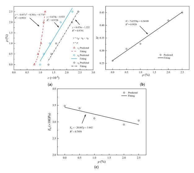
**Figure 8.** Influence of fiber volume fraction on the characteristic parameters: (a)  $\rho$ - $\varepsilon_a$ ,  $\varepsilon_h$ ,  $\varepsilon_b$  curves; (b) H- $\rho$  curve; (c)  $E_0$ - $\rho$  curve.
