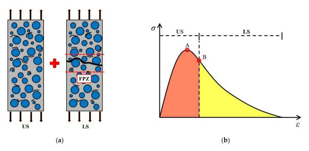
**Figure 1.** Two-stage feature of macroscopic mechanical behavior of concrete under uniaxial tension: (**a**) deformation-failure process; (**b**) typical nominal stress–strain curve.
