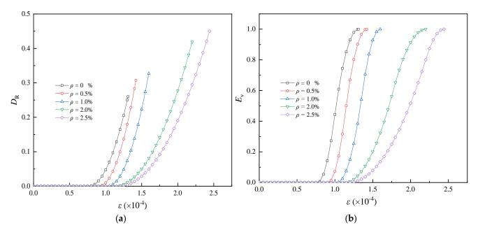
**Figure 9.** Evolution curves of damage variable and evolution factor: (a)  $D_R$ - $\varepsilon$  curves; (b)  $E_v$ - $\varepsilon$  curves.
