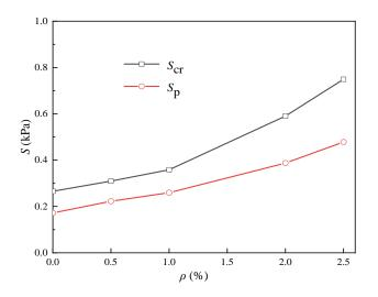
Figure 10. Influence of fiber volume fraction on the energy absorption capacity.
