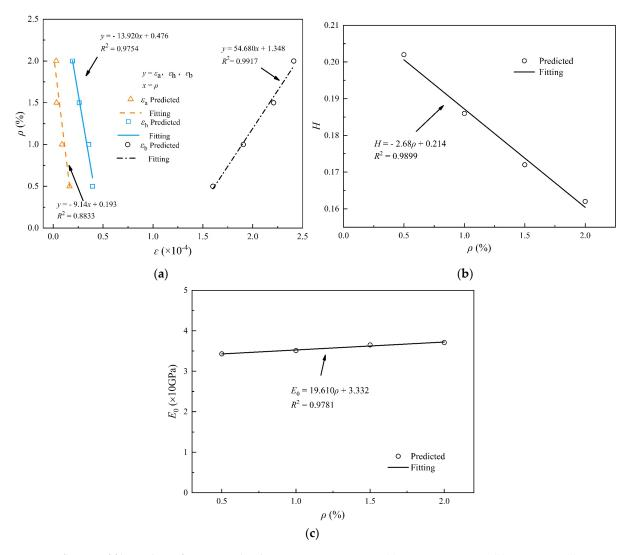
**Figure 12.** Influence of fiber volume fraction on the characteristic parameters: (a)  $\rho$ - $\varepsilon_a$ ,  $\varepsilon_h$ ,  $\varepsilon_b$  curves; (b) H- $\rho$  curve; (c)  $E_0$ - $\rho$  curve.
