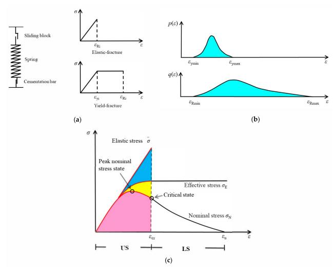
**Figure 2.** Mechanical behavior of concrete under uniaxial tension described by the Improved Parallel Bar System (IPBS): (a) micro bar and failure mode; (b) damage evolution process on meso-scale; (c) stress–strain curves on macro-scale.
