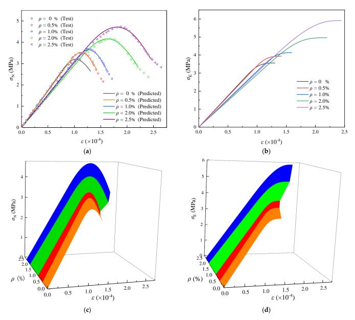
**Figure 7.** Stress–strain curves under uniaxial tension: (**a**) nominal stress–strain curve (Plan view); (**b**) effective stress–strain curve (Plan view); (**c**) envelope of the nominal stress–strain curve (3D view); (**d**) envelope of the effective stress–strain curve (3D view).
