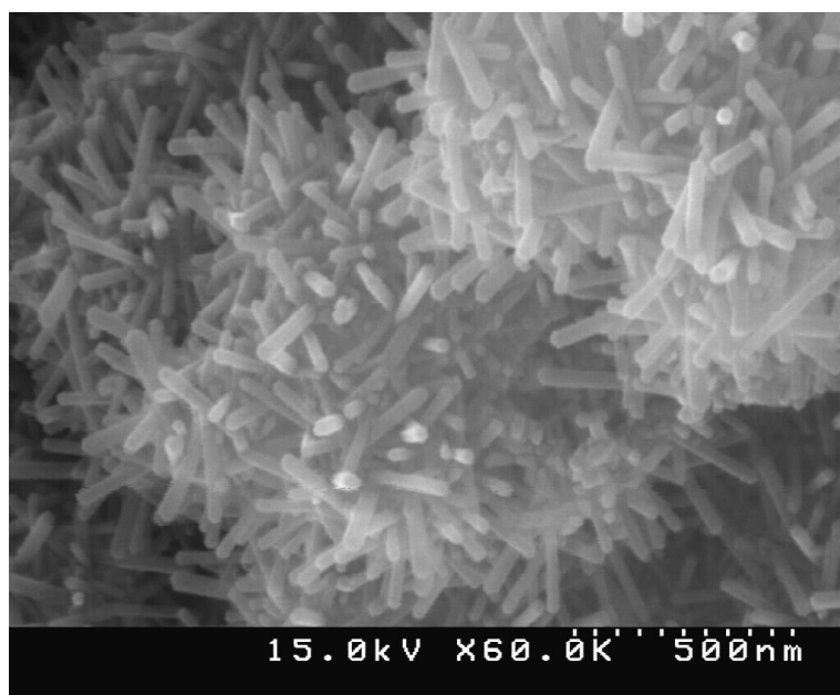
Figure 11. SEM image of \text{Bi}_2\text{O}_3 nanorods produced by thermolysis of nanostructure 1 at 170^\circ\text{C} .
