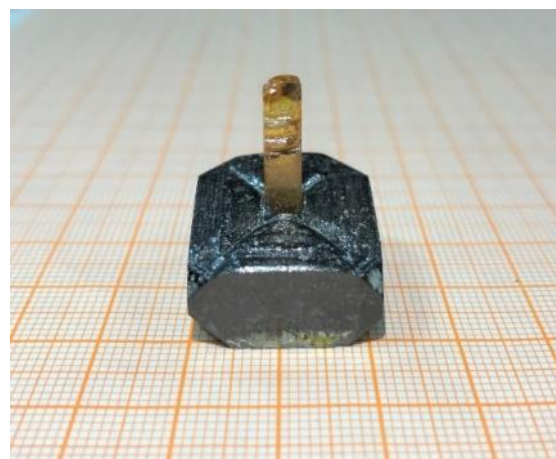
Figure 2. \text{Cr}:\text{TiTe}_3\text{O}_8 single crystal grown along [100] crystallographic axis.
