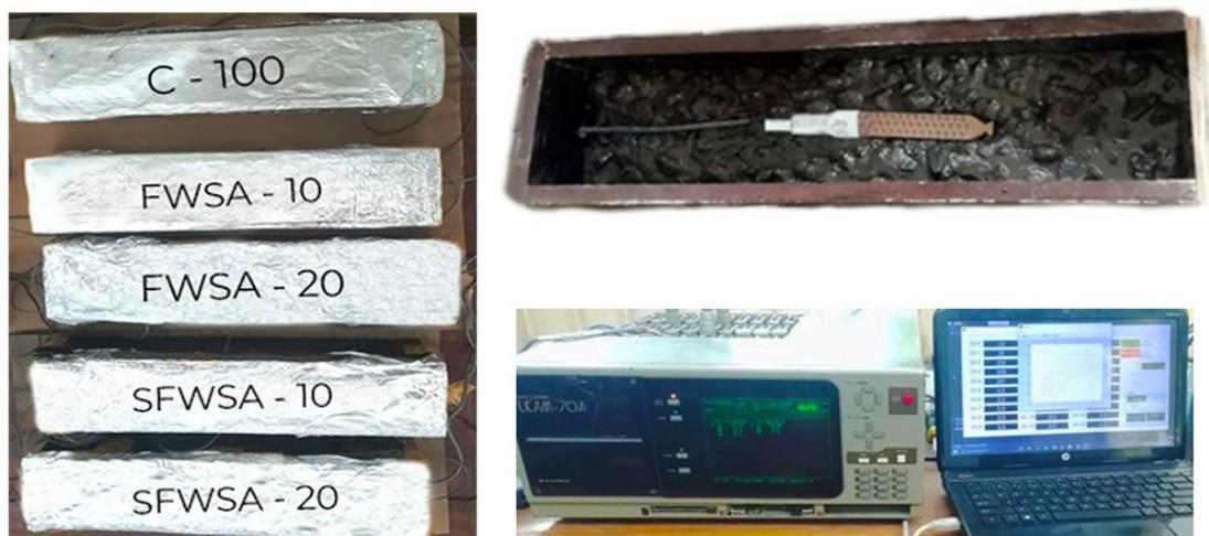
Figure 5. Experimental setup used for measurement of autogenous shrinkage of concrete beams.
