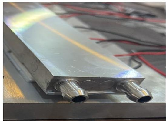
**Figure 3.** The practical configuration of the lower aluminum block with an M-shaped water channel.
