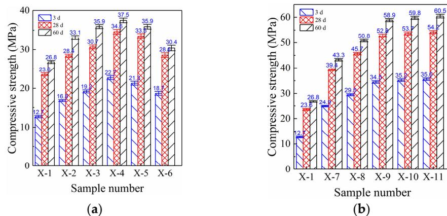
**Figure 1.** Regulation effect of sodium silicate on compressive strength (a) Solid sodium silicate excitation (b) Liquid sodium silicate excitation.
