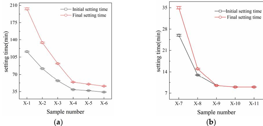
**Figure 2.** Regulation effect of sodium silicate on condensation behavior (a) Solid sodium silicate impact (b) Liquid sodium silicate impact.
