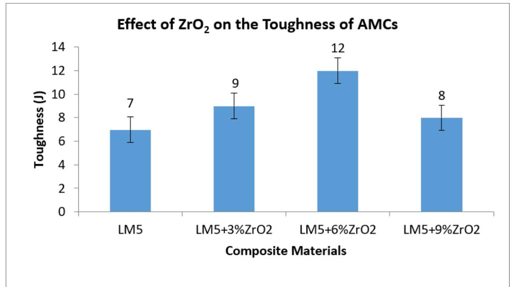
**Figure 14.** Impact strength of fabricated composites AMCs.
