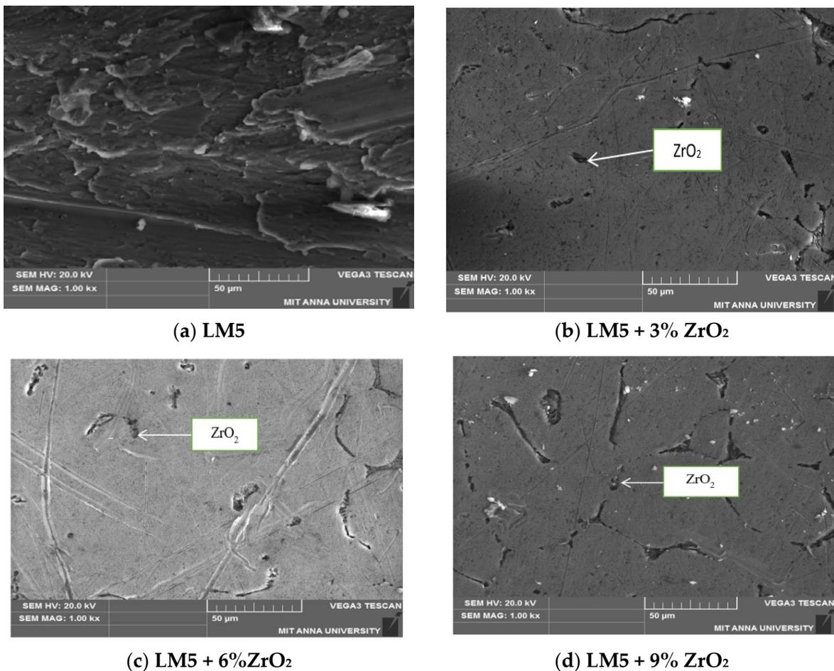
**Figure 4.** SEM images of LM5 and LM5/ $ZrO_2$  composites.
