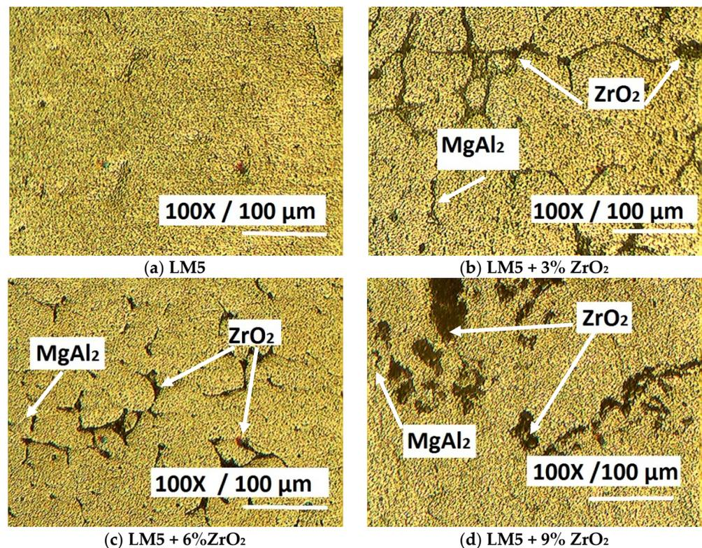
Figure 3. Micrographs of LM5 alloy and LM5/ZrO<sub>2</sub> composites.
