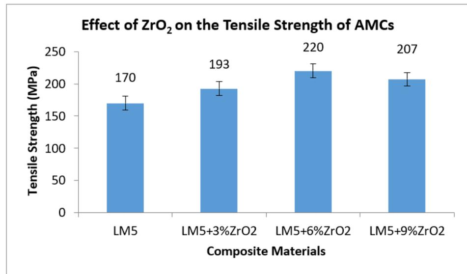
Figure 10. Effect of  $ZrO_2$  on the tensile strength of AMCs.
