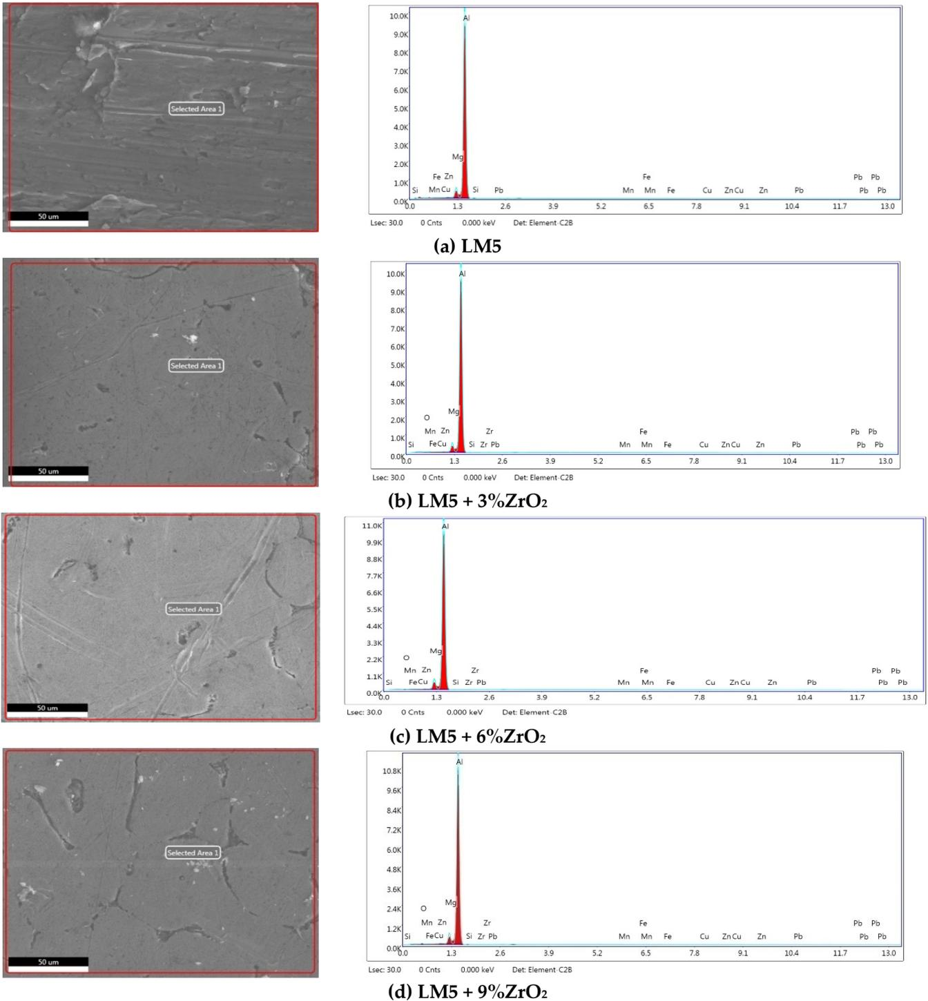
Figure 5. EDAX of LM5 and LM5/ $ZrO_2$  Composites.
