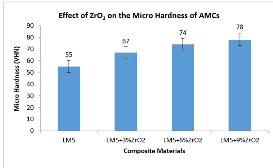
Figure 8. Effect of  $ZrO_2$  on the micro hardness of AMCs.
