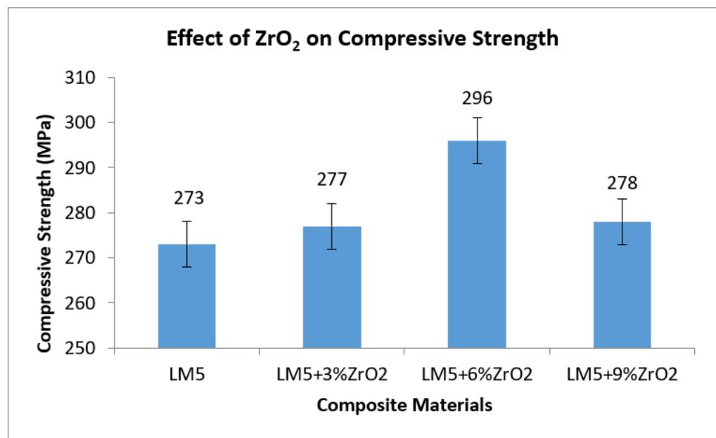
**Figure 12.** Effect of ZrO<sub>2</sub> on the compression strength of AMCs.
