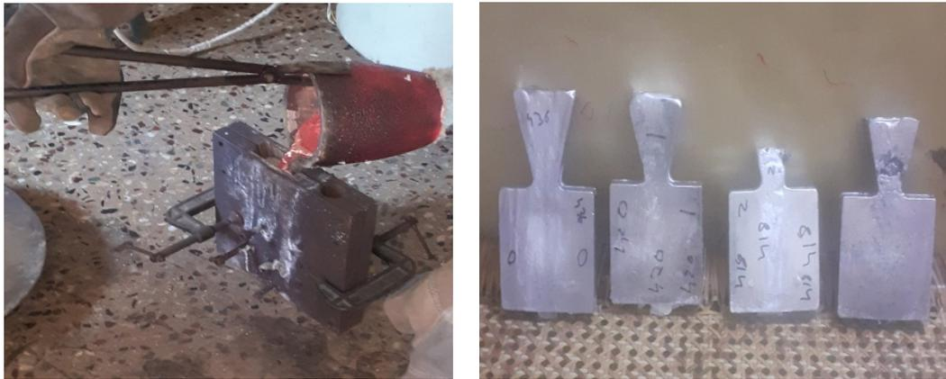
**Figure 2.** Pouring molten mixture into the preheated mold and fabricated composites.
