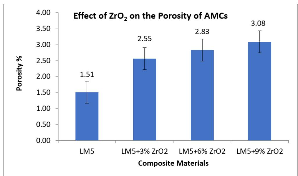
Figure 7. Effect of ZrO<sub>2</sub> on the porosity of AMCs.
