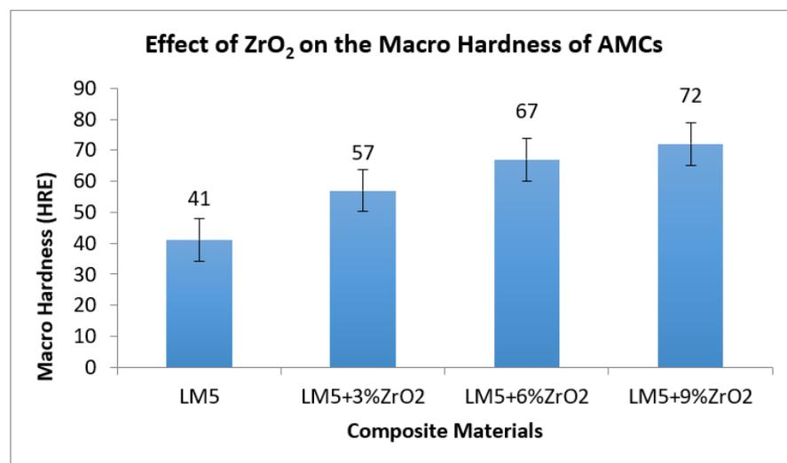
Figure 9. Effect of  $ZrO_2$  on the macro hardness of AMCs.
