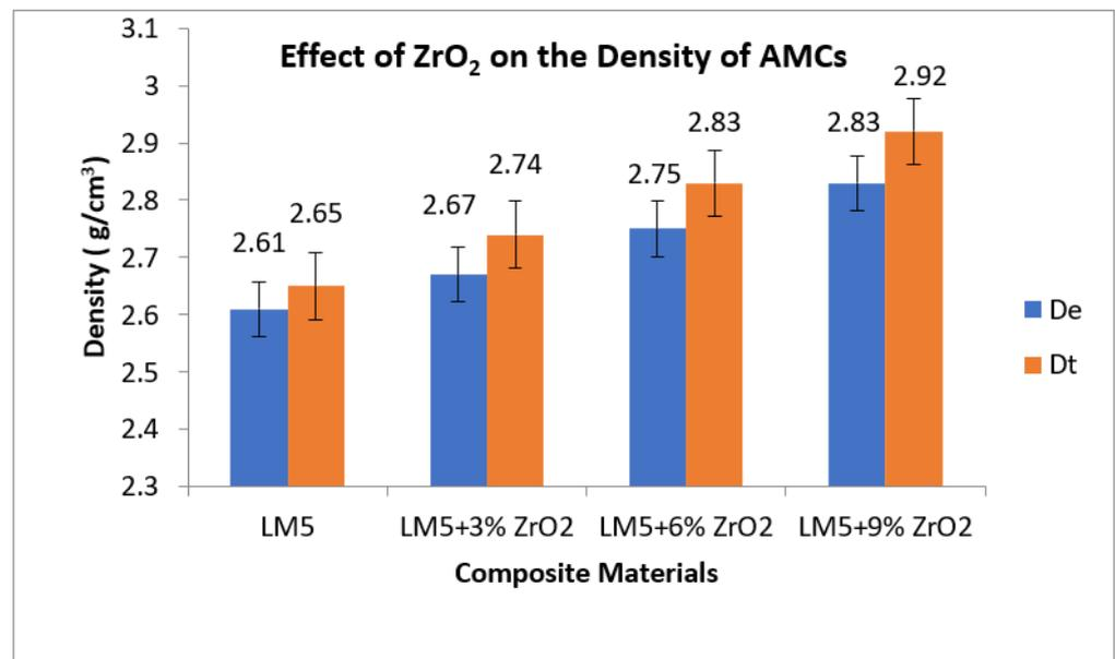
Figure 6. Effect of ZrO<sub>2</sub> on the density of AMCs.
