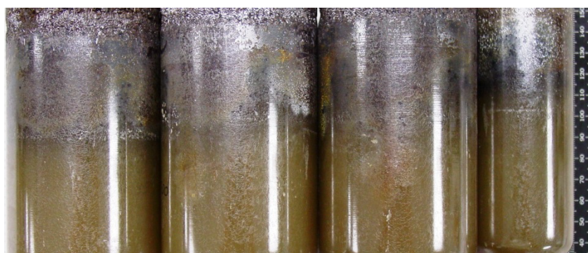
Figure 4. Seventy five-millimeter and 50-mm diameter \langle 001 \rangle -oriented PIN-PMN-PT crystals grown by the Bridgman process (courtesy of TRS Technologies, Inc., State College, PA, USA).
