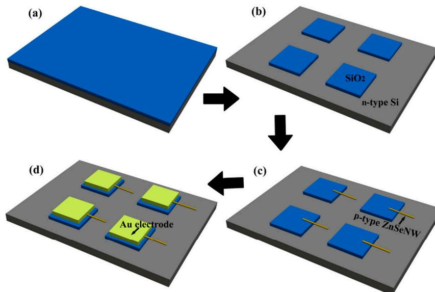
**Figure 8.** Schematic illustration of the fabrication process of ZnSeNW/Si p-n junction. Reproduced with permission from [44], Copyright 2016, Elsevier B.V.
