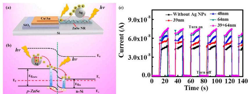
**Figure 13.** (a) Schematic illustration of the localized surface plasmon resonance excited electrons transfer from Ag nano particles to ZnSe nanoribbon. (b) Energy band diagram of ZnSe nanoribbon/Si heterojunction modified with Ag nanoparticles under light illumination. (c) Time response spectra of the devices without and with decoration of 39, 48, 64, and 39 + 64 nm Ag nanoparticles measured at zero voltage bias. Reproduced with permission from [45], Copyright 2016, IOP Publishing Ltd.
