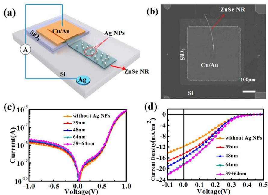
**Figure 11.** (a) Schematic illustration of ZnSe nanoribbon/Si heterojunction. (b) The top view SEM image of a single nanoribbon device. (c) Dark I-V characteristics of devices in the semi-logarithmic scale. (d) The J-V curves of devices embellished with different diameters of Ag nanoparticles measured under AM 1.5 G illumination at  $100 \text{ mW cm}^{-2}$ . Reproduced with permission from [45], Copyright 2016, IOP Publishing Ltd.
