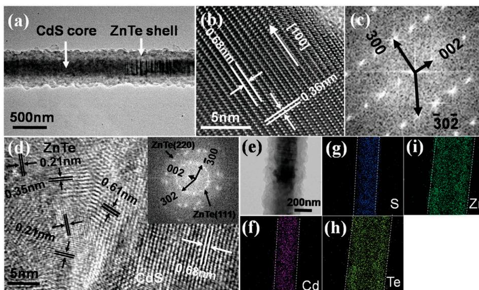
**Figure 1.** (a) TEM image of a CdS-ZnTe core-shell nanowire. (b) HRTEM image of the CdS nanowire; and (c) the corresponding FFT pattern. (d) High-magnification TEM image of a CdS-ZnTe core-shell nanowire. (e–i) TEM image of an individual core-shell nanostructure and the corresponding elemental mapping images for: Cd (f); S (g); Te (h); and Zn (i). Reproduced with permission from [25], Copyright 2015, The Royal Society of Chemistry.
