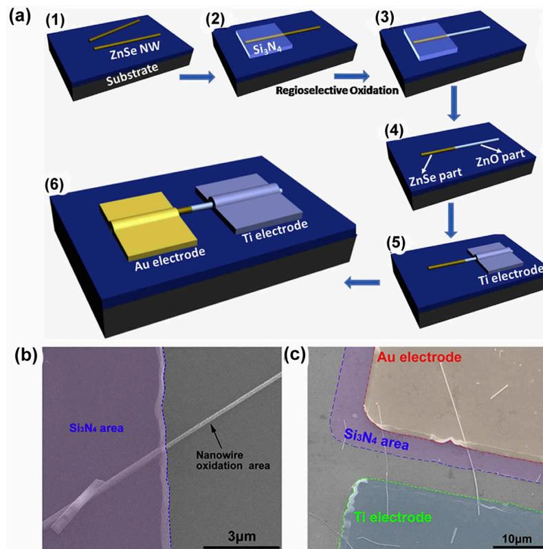
**Figure 6.** (a) Schematic illustration of the construction process of the ZnSe-ZnO axial p-n junction. (b) The SEM image of a nanowire whose bare part has already been oxidized. (c) The SEM image of a prepared ZnSe-ZnO nanowire axial p-n junction. Reproduced with permission from [39], Copyright 2015, Elsevier B.V.
