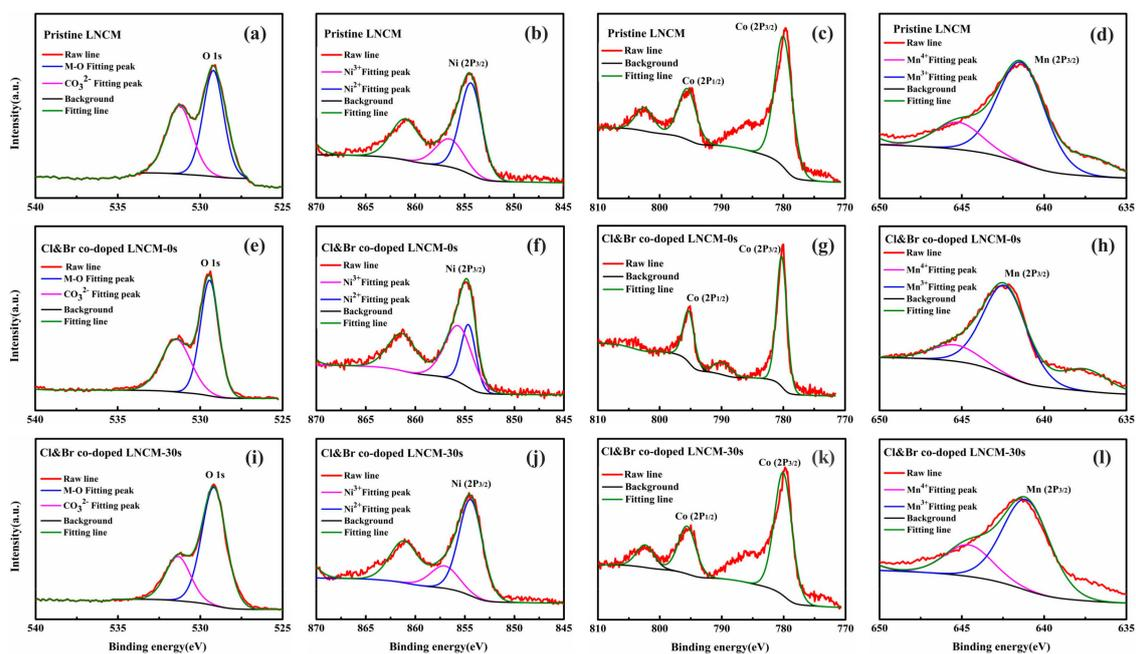
**Figure 3.** XPS spectra of (a) O 1s, (b) Ni  $2p_{3/2}$ , (c) Co  $2p_{3/2}$ , (d) Mn  $2p_{3/2}$  for Pristine LNCM; (e) O 1s, (f) Ni  $2p_{3/2}$ , (g) Co  $2p_{3/2}$ , (h) Mn  $2p_{3/2}$  for Cl&Br co-doped LNCM; (i) O 1s, (j) Ni  $2p_{3/2}$ , (k) Co  $2p_{3/2}$ , (l) Mn  $2p_{3/2}$  for Cl&Br co-doped LNCM being ion-etched for 30 s.
