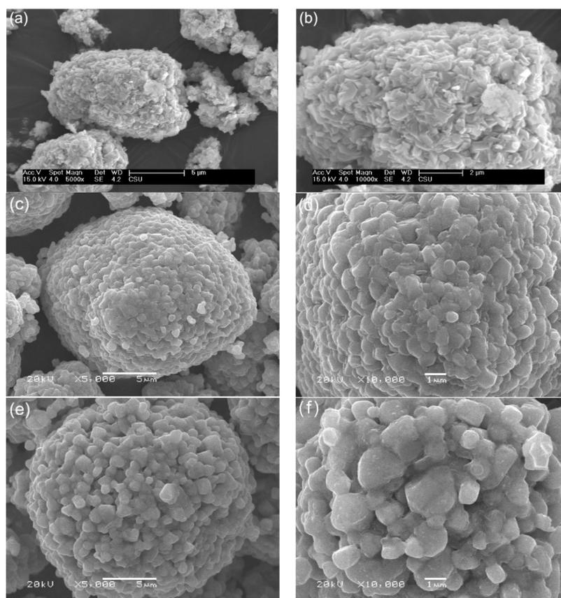
**Figure 1.** SEM images of the  $\text{Ni}_{1/3}\text{Co}_{1/3}\text{Mn}_{1/3}(\text{OH})_2$  precursor and the synthesized  $\text{LiNi}_{1/3}\text{Co}_{1/3}\text{Mn}_{1/3}\text{O}_2$  compounds: (a,b)  $\text{Ni}_{1/3}\text{Co}_{1/3}\text{Mn}_{1/3}(\text{OH})_2$  precursor; (c,d) Pristine LNCM; (e,f) Cl&Br co-doped LNCM.
