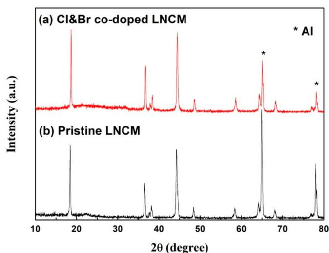
**Figure 7.** XRD patterns of the synthesized  $\text{LiNi}_{1/3}\text{Co}_{1/3}\text{Mn}_{1/3}\text{O}_2$  electrodes after 100 cycles: (a) Cl&Br co-doped LNCM; (b) Pristine LNCM.
