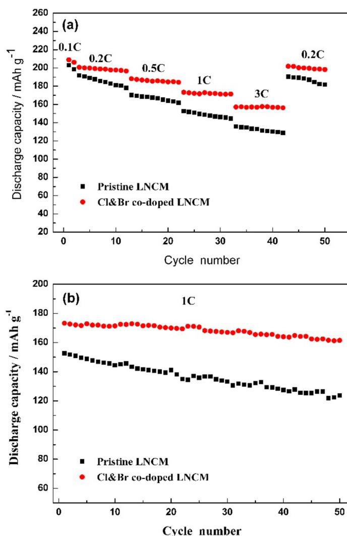
**Figure 5.** Rate capabilities (a) and cycling performance (b) of the synthesized  $\text{LiNi}_{1/3}\text{Co}_{1/3}\text{Mn}_{1/3}\text{O}_2$  compounds.
