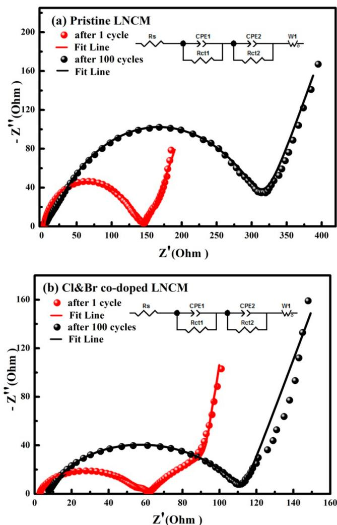
**Figure 8.** Electrochemical impedance spectra of the synthesized  $\text{LiNi}_{1/3}\text{Co}_{1/3}\text{Mn}_{1/3}\text{O}_2$  electrodes after different cycles: (a) Pristine LNCM; (b) Cl&Br co-doped LNCM.
