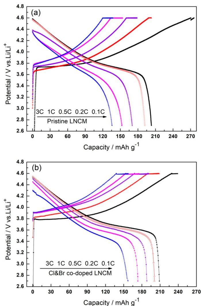
**Figure 4.** Initial charge and discharge capacities of the synthesized  $\text{LiNi}_{1/3}\text{Co}_{1/3}\text{Mn}_{1/3}\text{O}_2$  compounds at 0.1~3C: (a) Pristine LNCM; (b) Cl&Br co-doped LNCM.
