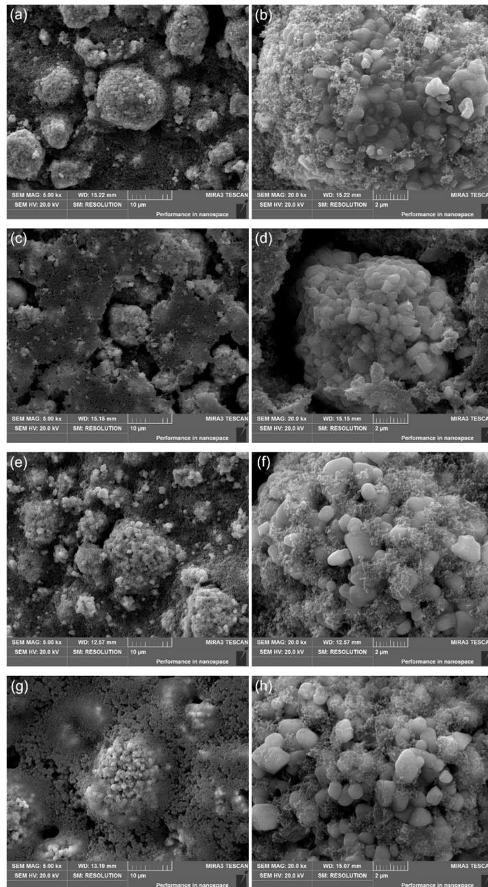
**Figure 6.** SEM images of the synthesized  $\text{LiNi}_{1/3}\text{Co}_{1/3}\text{Mn}_{1/3}\text{O}_2$  electrodes after cycling (100 cycles): (a,b) Pristine LNCM before cycling; (c,d) Pristine LNCM after cycling; (e,f) Cl&Br co-doped LNCM before cycling; (g,h) Cl&Br co-doped LNCM after cycling.
