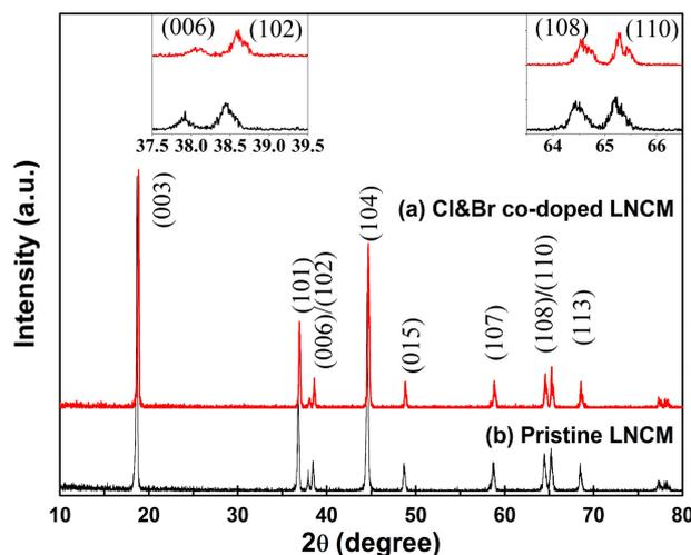
**Figure 2.** XRD patterns of the synthesized  $\text{LiNi}_{1/3}\text{Co}_{1/3}\text{Mn}_{1/3}\text{O}_2$  compounds: (a) Cl&Br co-doped LNCM; (b) Pristine LNCM.
