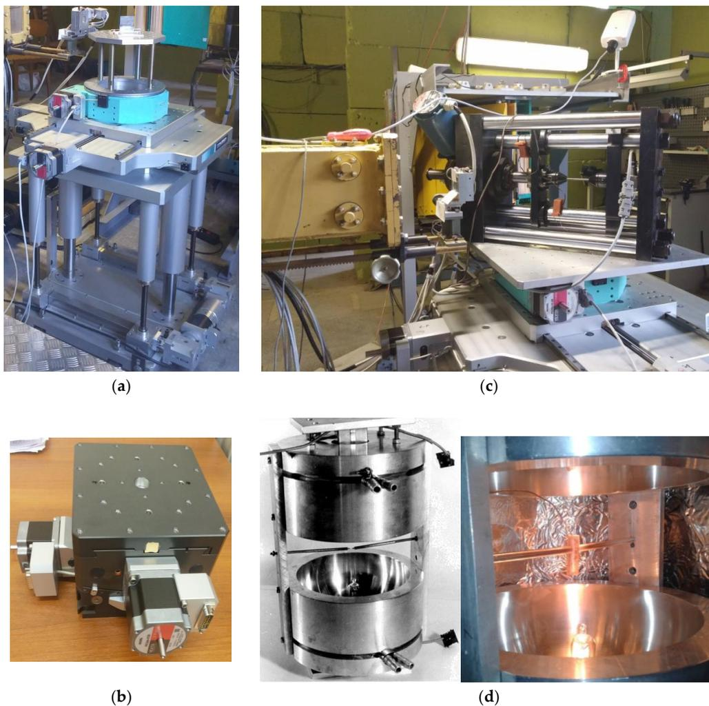
**Figure 13.** (a) Four-axis HUBER goniometer for precise sample positioning (max. load 300 kg); (b) Additional goniometer head with  $\pm 15^\circ$ -tilt; (c) Uniaxial mechanical loading machine LM-29 ( $F_{max} = 29$  kN,  $T_{max} = 800$  °C) installed on the HUBER goniometer during the experiment; (d) Water-cooled mirror furnace ( $P = 1$  kW,  $T_{max} = 1000$  °C). A sample with a thermocouple heated during the experiment is shown.
