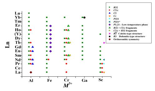
**Figure 1.** Space groups for the compounds with the general composition  $LnM_3(BO_3)_4$  with the  $M^{3+}$  = Al, Fe, Cr, Ga, Sc (according to the literature data given in Table 1).
