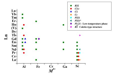
**Figure 2.** Space groups for the single crystals with the general composition  $LnM_3(BO_3)_4$  with the  $M^{3+} = Al$ , Fe, Ga, Sc (according to the literature data on X-ray diffraction experiments given in Table 1).
