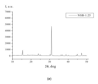
**Figure 12.** Theoretical diffraction patterns for the (a) huntite structure (space group R32), (b) superstructure of the huntite structure (space group P321), (c) structure with the space group  $P3_121$ ; Experimental diffraction patterns of powdered single crystals (space group P321): (c)  $Pr_{1.1}Sc_{2.9}(BO_3)_4$  (PSB–1.1), (d)  $NdSc_3(BO_3)_4$  (NSB–1.0), (e)  $Nd_{1.25}Sc_{2.75}(BO_3)_4$  (NSB–1.25).
