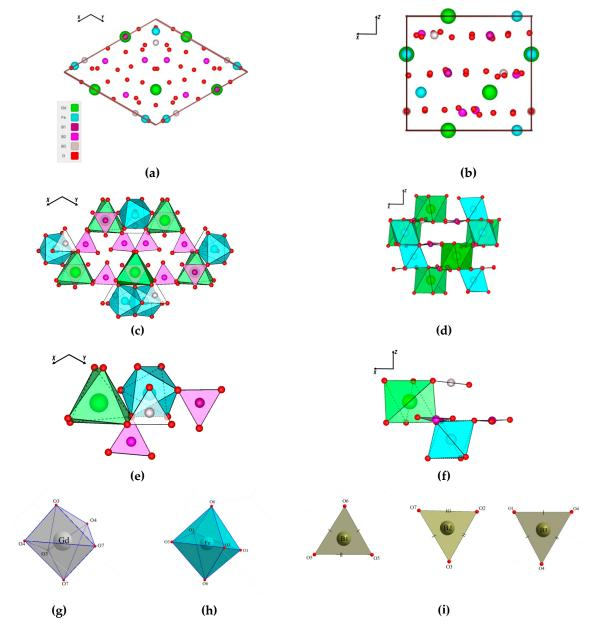
**Figure 13.** The unit cell of the  $GdFe_3(BO_3)_4$  structure (space group  $P3_121$ ) projected onto the (a) XY and (b) XZ planes; Combination of the coordination polyhedra projected onto the (c) XY and (d) XZ planes; Combination of selected coordination polyhedra projected onto the (e) XY and (f) XZ planes; Coordination polyhedra for the (g) Gd, (h) Fe, (i) B1-B3.
