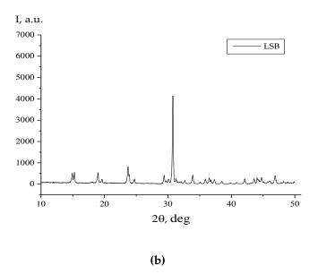
**Figure 10.** (a) Theoretical and (b) experimental diffraction patterns for the  $\alpha$  - LaSc<sub>3</sub>(BO<sub>3</sub>)<sub>4</sub> structure (space group C2/c).
