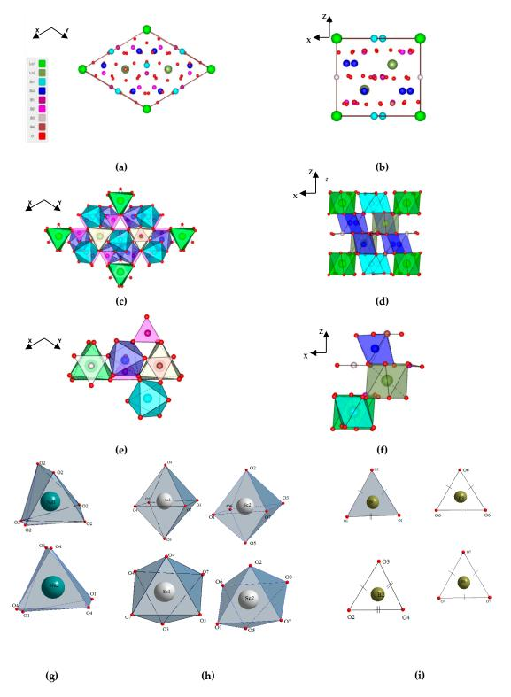
**Figure 5.** The unit cell of the  $NdSc_3(BO_3)_4$  (NSB–1.0) structure (space group *P*321) projected onto the (a) XY and (b) XZ planes; Combination of the coordination polyhedra projected onto the (c) XY and (d) XZ planes; Combination of selected coordination polyhedra projected onto the (e) XY and (f) XZ planes; Coordination polyhedra for the (g) Nd1 and Nd2, (h) Sc1 and Sc2, (i) B1–B4.
