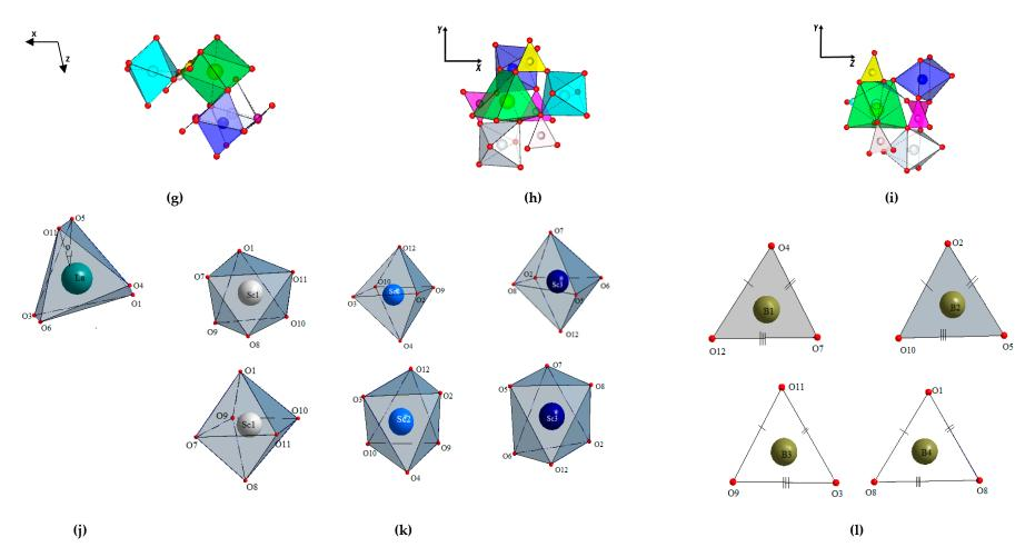
**Figure 8.** The unit cell of the  $LnM_3(BO_3)_4$  structure (space group Cc) projected onto the (**a**) XZ, (**b**) XY, (**c**) YZ planes; Combination of the coordination polyhedra projected onto the (**d**) XZ, (**e**) XY, (**f**) YZ planes; Combination of selected coordination polyhedra projected onto the (**g**) XZ, (**h**) XY, (**i**) YZ planes; Coordination polyhedra for the (**j**) Ln, (**k**) M1-M3, (**l**) B1-B4.
