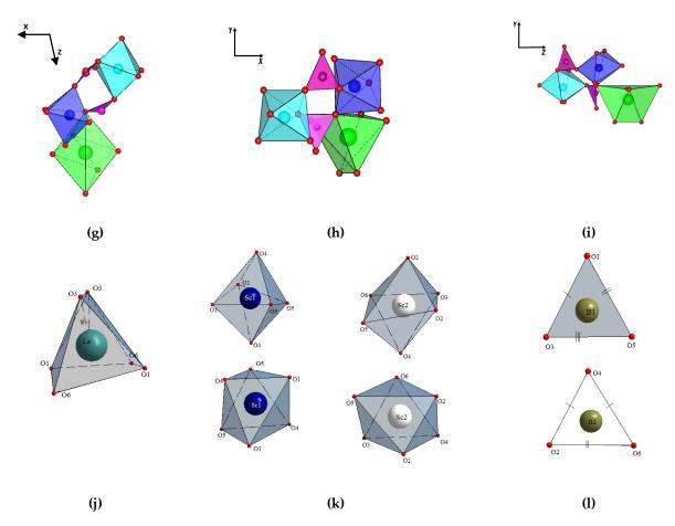
**Figure 7.** The unit cell of the  $LnM_3(BO_3)_4$  structure (space group C2/c) projected onto the (a) XZ, (b) XY, (c) YZ planes; Combination of the coordination polyhedra projected onto the (d) XZ, (e) XY, (f) YZ planes; Combination of selected coordination polyhedra projected onto the (g) XZ, (h) XY, (i) YZ planes; Coordination polyhedra for the (j) Ln, (k) M1 and M2, (l) B1 and B2.
