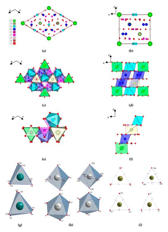
**Figure 6.** The unit cell of the  $NdSc_3(BO_3)_4$  (NSB-1.25) structure (space group P321) projected onto the (a) XY and (b) XZ planes; Combination of the coordination polyhedra projected onto the (c) XY and (d) XZ planes; Combination of selected coordination polyhedra projected onto the (e) XY and (f) XZ planes; Coordination polyhedra for the (g) Nd1 and Nd2, (h) Sc1 and Sc2, (i) B1-B4.
