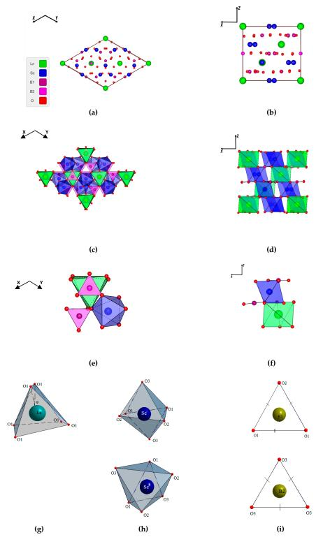
**Figure 3.** The unit cell of the  $LnM_3(BO_3)_4$  structure (space group R32) projected onto the (a) XY and (b) XZ planes; Combination of the coordination polyhedra projected onto the (c) XY and (d) XZ planes; Combination of selected coordination polyhedra projected onto the (e) XY and (f) XZ planes; Coordination polyhedra for the (g) Ln, (h) M, (i) B1 and B2.
