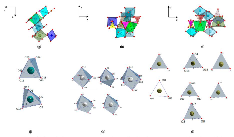
**Figure 9.** The unit cell of the  $LnM_3(BO_3)_4$  structure (space group C2) projected onto the (**a**) XZ, (**b**) XY, (**c**) YZ planes; Combination of the coordination polyhedra projected onto the (**d**) XZ, (**e**) XY, (**f**) YZ planes; Combination of selected coordination polyhedra projected onto the (**g**) XZ, (**h**) XY, (**i**) YZ planes; Coordination polyhedra for the (**j**) Ln1 and Ln2, (**k**) M1-M5, (**l**) B1-B7.
