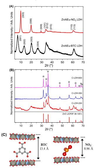
**Figure 2.** Powder X-ray diffraction patterns of (**A**) the as-prepared ZnAlEu LDHs and (**B**) ZnAlEu–NO<sub>3</sub> LDHs calcined at 200 °C (C-LDH-200), 350 °C (C-LDH-350), and 600 °C (C-LDH-600). Starred peaks are related to the formation of a ZnO-like phase. The diffractogram of ZnO is shown for comparison. (**C**) Intercalation scheme and basal spacing for LDHs with 1,3,5-benzenetricarboxilate (BTC) and NO<sub>3</sub><sup>-</sup> [30].
