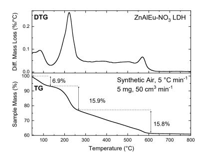
Figure 3. Thermogravimetric analysis of the ZnAlEu–NO<sub>3</sub> LDHs.
