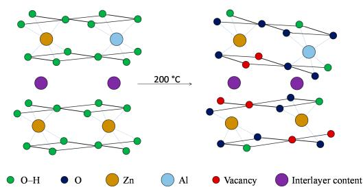
Figure 4. Schematic overview of the dehydroxylation of LDHs at low temperatures.
