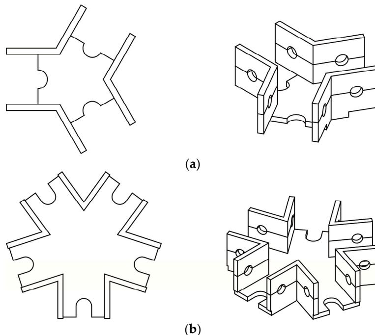
**Figure 9.** Plan view and 3D view of the base of novel joints with bevel gears: (a) Connected to three link members; (b) connected to five link members.
