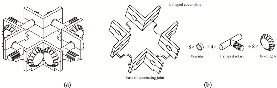
**Figure 7.** Design of a joint with four pairs of bevel gears and connected to  $n_1 = 4$  link members: (a) Sketch of the joint model; (b) basic components, including base, cover plate, bearing, rotary, and bevel gears.
