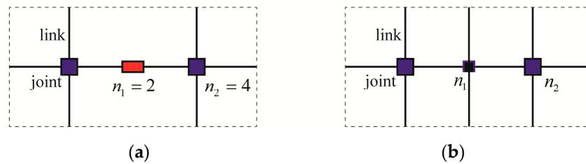
**Figure 1.** Unit cells of deployable structures assembled by different types of joints, which are designed to respectively connect to  $n_1$  and  $n_2$  links: (a)  $n_1 = 2$ , and  $n_2 = 4$ ; (b)  $n_1 = n_2 = 4$ .
