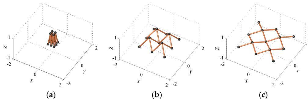
**Figure 3.** Motion of a deployable structure assembled by  $2 \times 2$  basic units, with  $n_1 = n_2 = 4$ : (a) Folded configuration; (b) partially deployed configuration; (c) deployed configuration.
