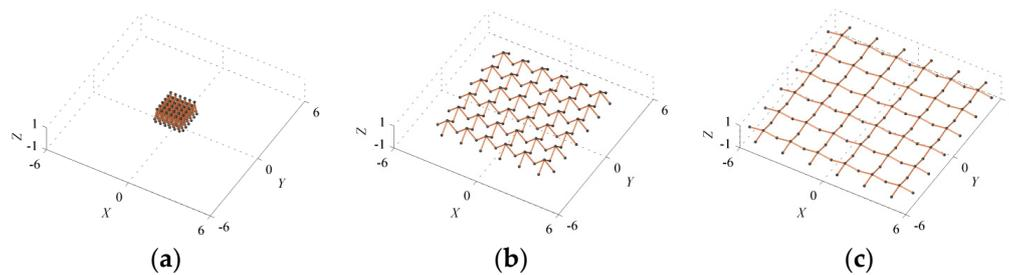
**Figure 4.** Motion of a deployable structure assembled by  $6 \times 6$  basic units, with  $n_1 = 2$  and  $n_2 = 4$ : (a) Folded configuration; (b) partially deployed configuration; (c) deployed configuration.
