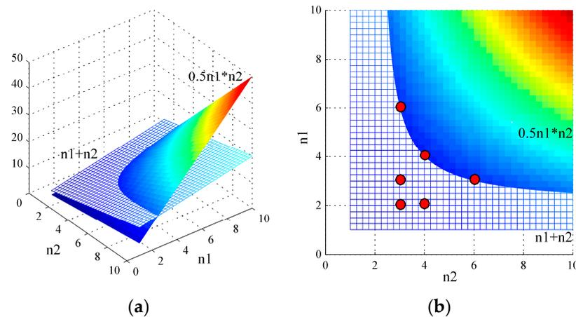
**Figure 2.** Feasible solutions to the compatibility conditions of the members given by Equations (3) and (4): (a) Three-dimensional (3D) view; (b) typical solutions marked by the dots.
