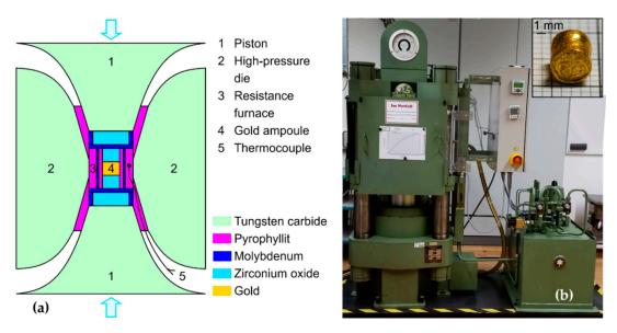
**Figure 2.** Schematic cross-section (**a**) of the high-pressure die and the pressure cell of the belt press at the Max-Planck-Institute for Solid State Research (Stuttgart, Germany), and the gold ampoule after treatment ((**b**), top).
