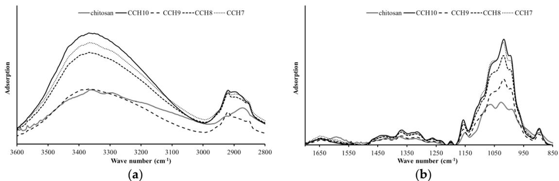
**Figure 3.** FT-IR spectra of the CCH films in the range of  $3600$  to  $2800\text{ cm}^{-1}$  (a) and  $1700$  to  $850\text{ cm}^{-1}$  (b).
