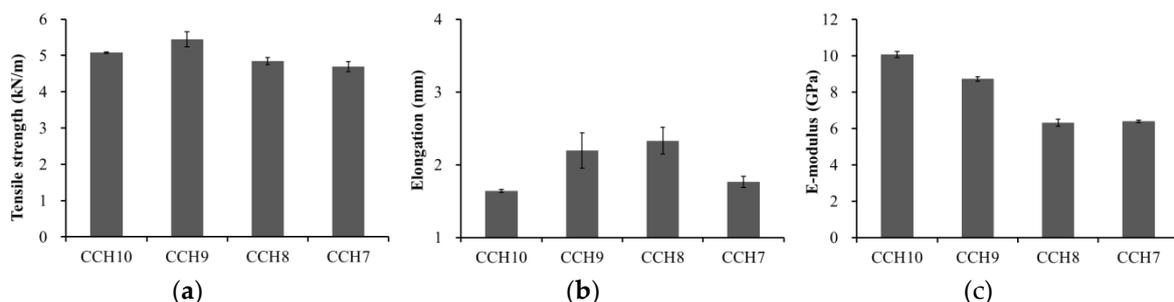
**Figure 4.** Tensile strength (a), elongation (b), and E-modulus (c) of the CCH films.
