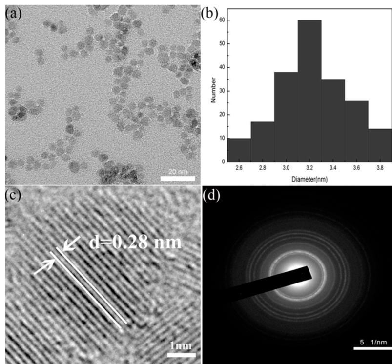
**Figure 1.** (a) TEM image of ZnOQD, (b) diameter distribution histogram calculated by TEM, (c) enlarged HRTEM (high-resolution transmission electron microscope) image of ZnOQD, (d) SAED (selected area electron diffraction) pattern of ZnOQD.
