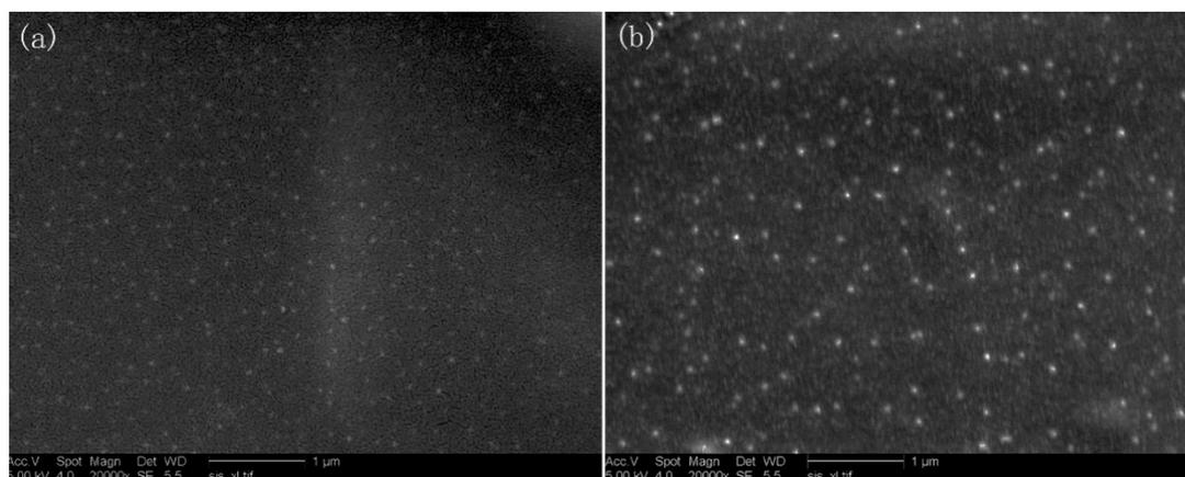
**Figure 3.** SEM images of (a): 5 wt % QD-CMC and (b): 15 wt % QD-CMC composites.
