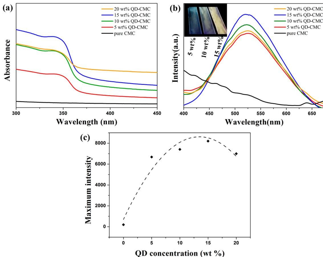
**Figure 6.** (a) UV-vis spectra and (b) photoluminescence spectra ( $\text{ex} = 350 \text{ nm}$ ) of pure CMC and composites. Inset in (b) is digital photographs of ZnOQD/CMC nanocomposite films under 365 nm UV lamp. (c) Maximum intensity of the photoluminescence spectra of ZnOQD/CMC nanocomposite films with different ZnOQD concentrations.
