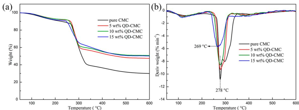
**Figure 5.** Thermogravimetric analysis (TGA) and differential thermogravimetry (DTG) curves of CMC and composites, (a) TGA curves; and (b) DTG curves.
