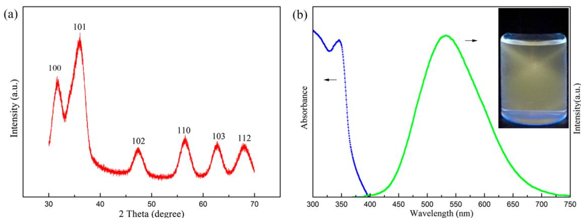
**Figure 2.** (a) XRD pattern of ZnOQD, (b) UV-vis and photoluminescence spectra of ZnOQD.
