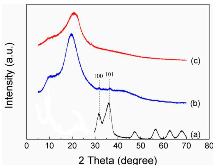
**Figure 4.** XRD patterns of (a): ZnOQD (b): 10 wt % QD-CMC composites and (c): pure CMC.
