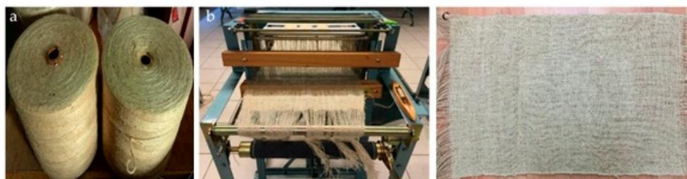
**Figure 1.** (a) Kenaf yarn with 500tex linear density wound on cylindrical bobbins; (b) hand loom used in the weaving process; (c) kenaf woven fabric.
