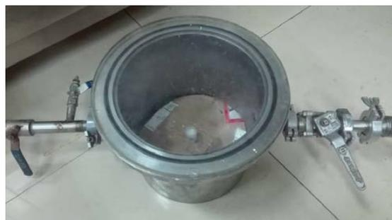
**Figure 1.** Vacuum tank used for eliminating air bubbles.
