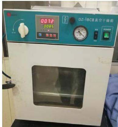
Figure 2. DZ-1BCII vacuum-drying oven.
