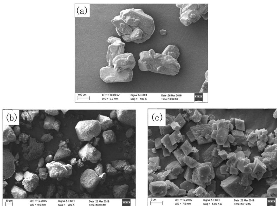
**Figure 1.** SEM photographs of (a) sodium tetraborate decahydrate, (b) ammonium pentaborate, and (c) zinc borate.
