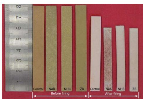
**Figure 6.** Surface morphology of ceramizable MVQ/HNT composites and corresponding ceramic residues obtained from the pyrolysis products of the composites with the addition of different borates.
