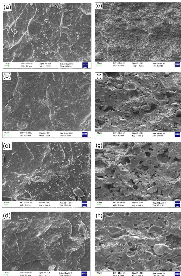
**Figure 8.** Morphology of tensile fracture surfaces of (a) the control and ceramizable, (b) NaB, (c) NHB, and (d) ZB composites and impact fracture surfaces of (e) the ceramic residue obtained from the control composite and the ceramic ones derived from the decomposition of the (f) NaB, (g) NHB, and (h) ZB composites, respectively.
