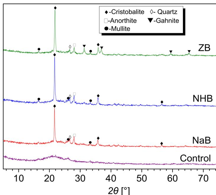
**Figure 9.** XRD spectra of the ceramic residues obtained from the MVQ/HNT composites with the addition of different borates.
