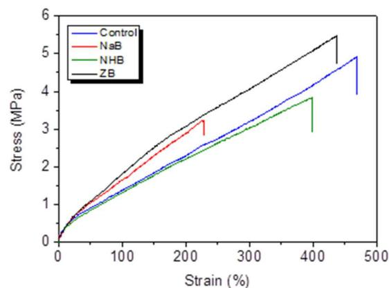
**Figure 3.** Tensile stress–strain curves of ceramizable MVQ/HNT composites with the addition of different borates.
