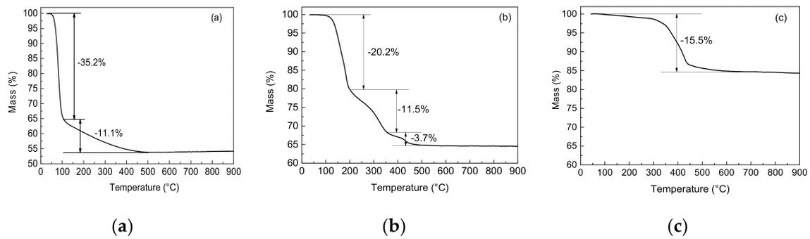
**Figure 2.** TGA curves of (a) sodium tetraborate decahydrate, (b) ammonium pentaborate, and (c) zinc borate.
