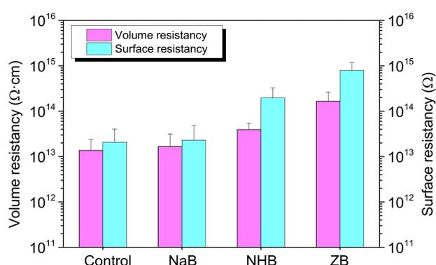
**Figure 4.** Electrical insulation properties of ceramizable MVQ/HNT composites with the addition of different borates.
