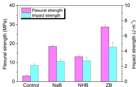
**Figure 7.** Effect of three borates on the flexural and impact strength of ceramic residues.
