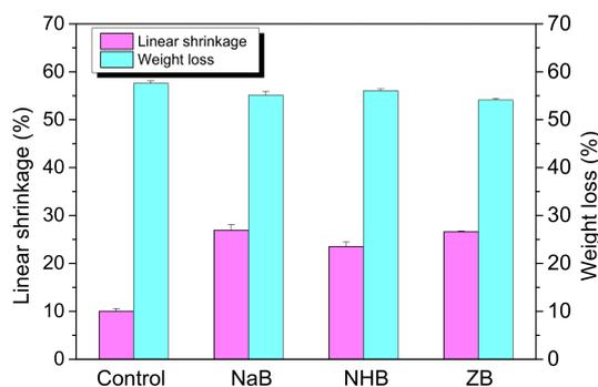
**Figure 5.** Linear shrinkage and weight loss of the ceramic residues by incorporation of different borates.
