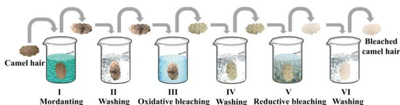
Figure 1. Simulation of experimental procedures.
