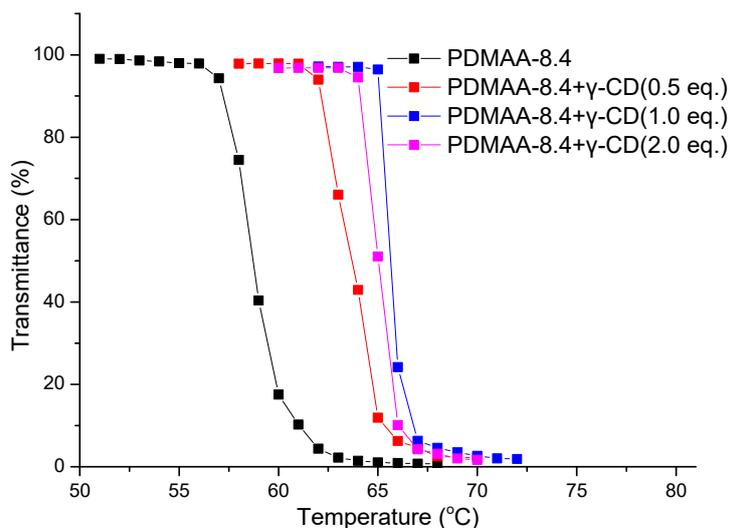
**Figure S10.** Transmittance as function of temperature for 5 g/L PDMAA-8.4 copolymers aqueous solution in the presence of different amount of  $\gamma$ -CD.
