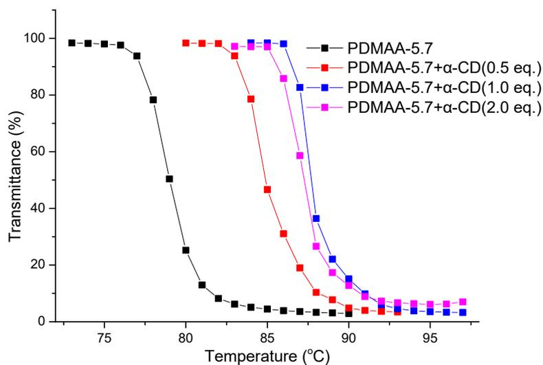
**Figure S2.** Transmittance as function of temperature for 5 g/L PDMAA-5.7 copolymers aqueous solution in the presence of different amount of  $\alpha$ -CD.
