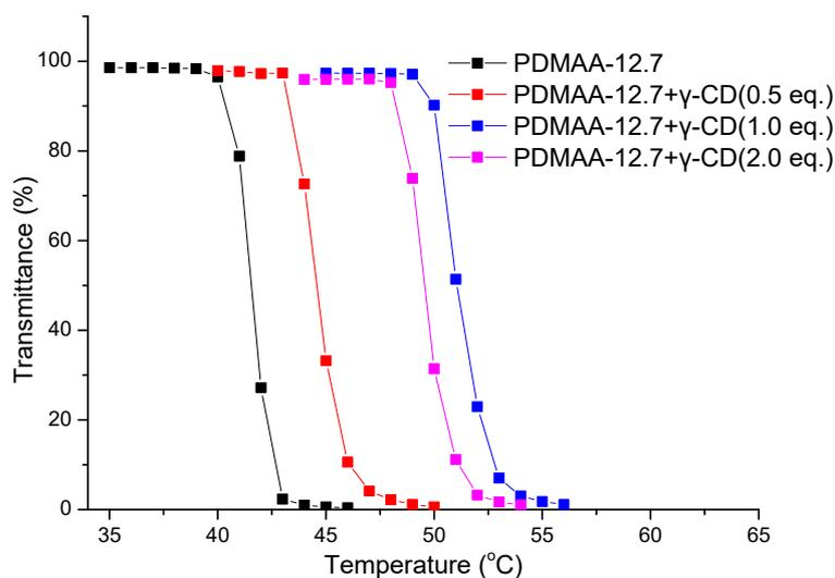
**Figure S13.** Transmittance as function of temperature for 5 g/L PDMAA-12.7 copolymers aqueous solution in the presence of different amount of  $\gamma$ -CD.
