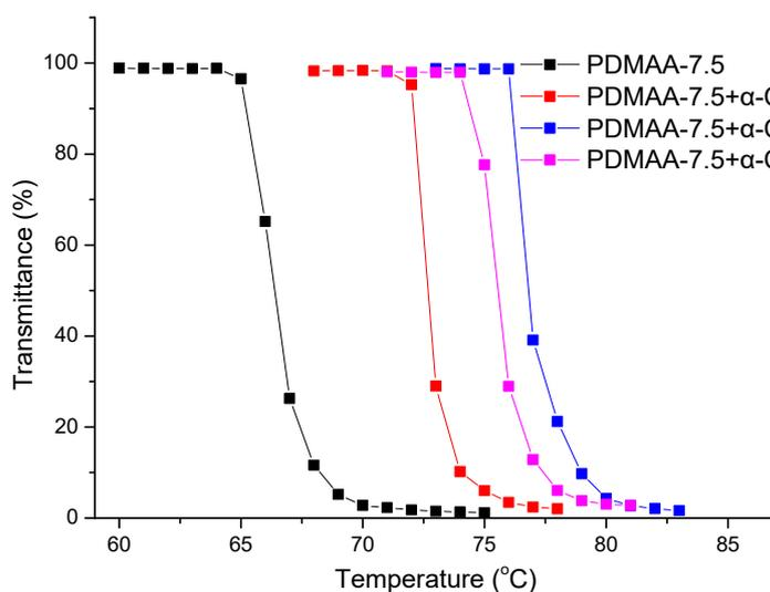
**Figure S5.** Transmittance as function of temperature for 5 g/L PDMAA-7.5 copolymers aqueous solution in the presence of different amount of  $\alpha$ -CD.
