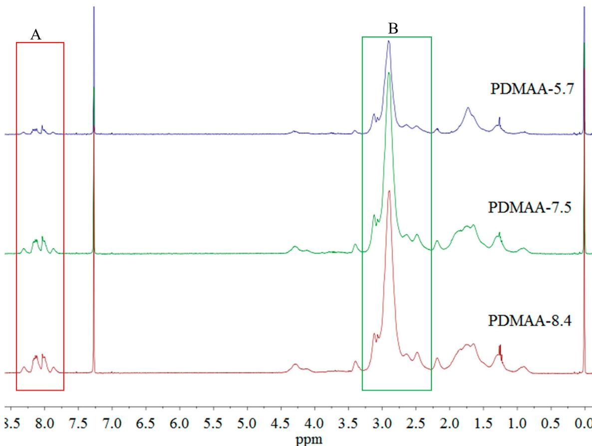
Figure S1. <sup>1</sup>H NMR spectra of PDMAA-5.7, PDMAA-7.5 and PDMAA-8.4 in CDCl<sub>3</sub>.
