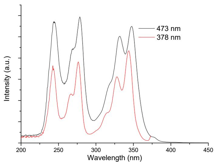
**Figure S16.** Excitation spectra of 10 µg/L PDMAA-12.7 copolymers aqueous solution with equivalent β-CD. Emission wavelength was fixed at 473 nm (black curve) and 378 nm (red curve) respectively.
