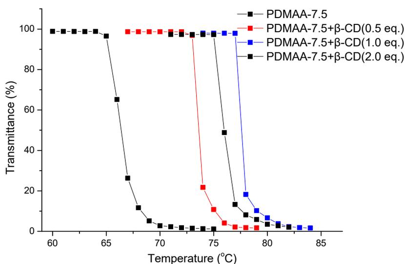
**Figure S6.** Transmittance as function of temperature for 5 g/L PDMAA-7.5 copolymers aqueous solution in the presence of different amount of  $\beta$ -CD.
