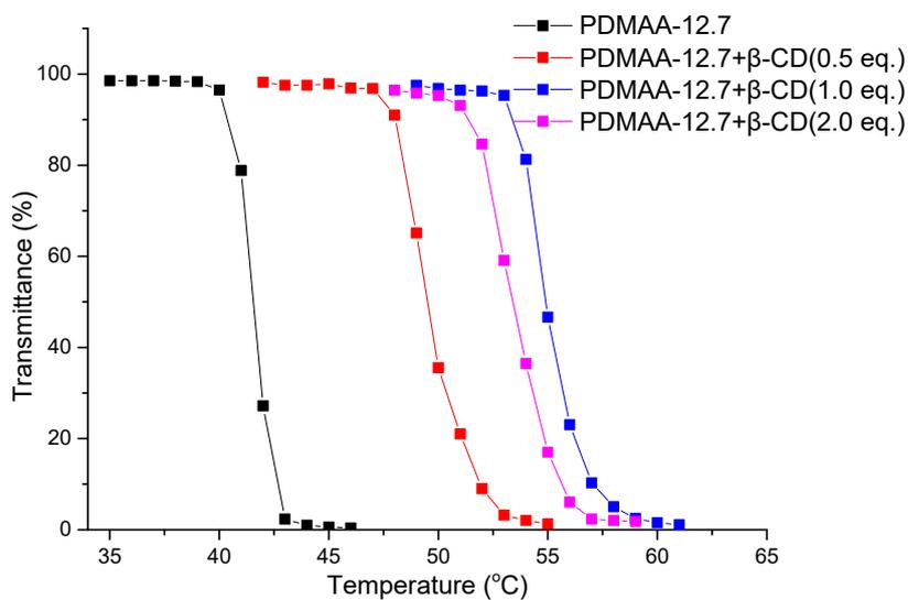
**Figure S12.** Transmittance as function of temperature for 5 g/L PDMAA-12.7 copolymers aqueous solution in the presence of different amount of  $\beta$ -CD.
