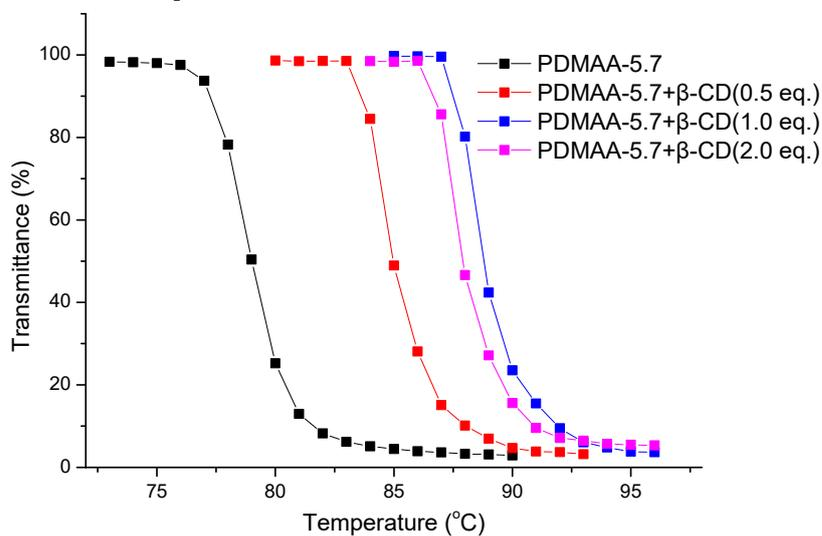
**Figure S3.** Transmittance as function of temperature for 5 g/L PDMAA-5.7 copolymers aqueous solution in the presence of different amount of  $\beta$ -CD.
