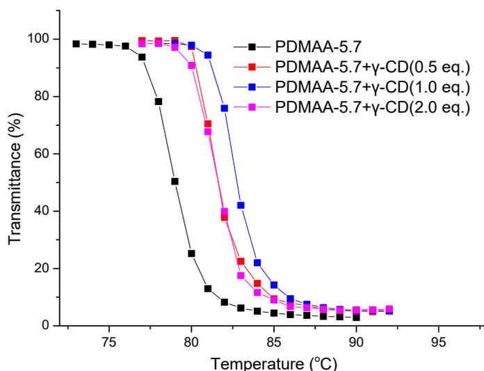
**Figure S4.** Transmittance as function of temperature for 5 g/L PDMAA-5.7 copolymers aqueous solution in the presence of different amount of  $\gamma$ -CD.
