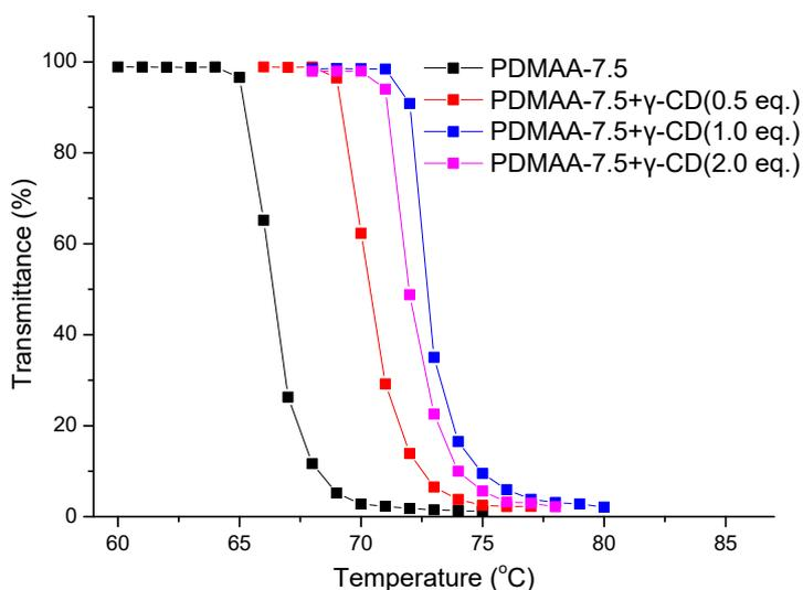
**Figure S7.** Transmittance as function of temperature for 5 g/L PDMAA-7.5 copolymers aqueous solution in the presence of different amount of  $\gamma$ -CD.
