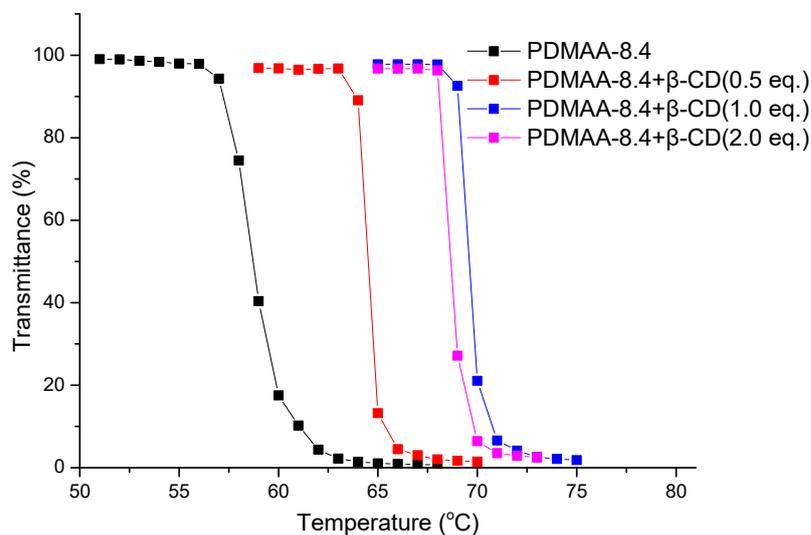
**Figure S9.** Transmittance as function of temperature for 5 g/L PDMAA-8.4 copolymers aqueous solution in the presence of different amount of  $\beta$ -CD.
