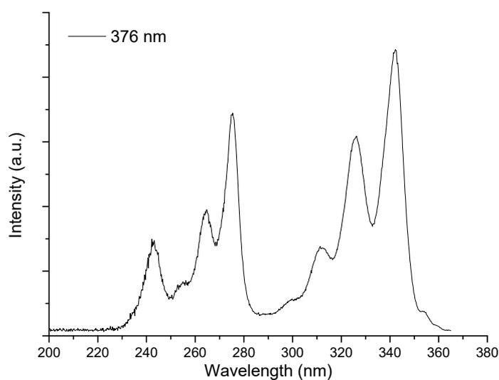
**Figure S18.** Excitation spectrum of 10 µg/L PDMAA-12.7 copolymers in ethanol. Emission wavelength was fixed at 376 nm.
