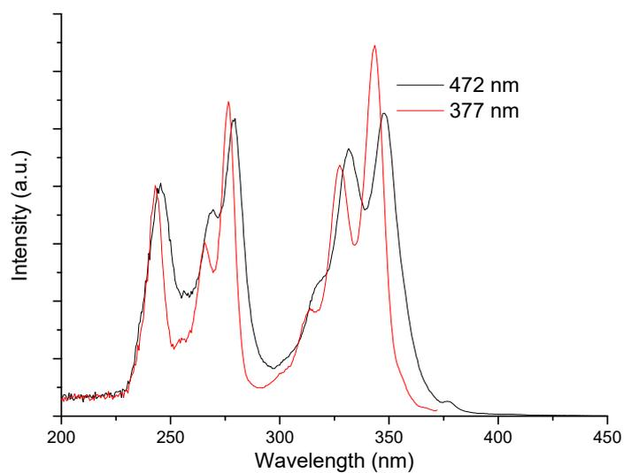
**Figure S15.** Excitation spectra of 10 µg/L PDMAA-12.7 copolymers aqueous solution with equivalent α-CD. Emission wavelength was fixed at 472 nm (black curve) and 377 nm (red curve) respectively.
