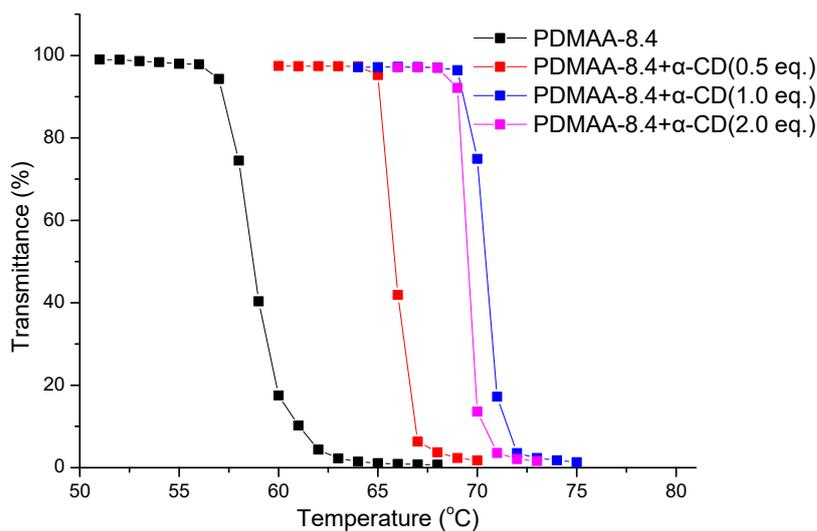
**Figure S8.** Transmittance as function of temperature for 5 g/L PDMAA-8.4 copolymers aqueous solution in the presence of different amount of  $\alpha$ -CD.
