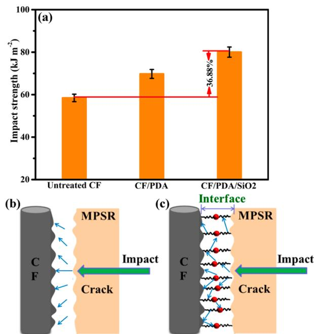
**Figure 7.** Impact testing results of composites and schematic of impact testing of composites reinforced with (a) untreated CF and (b) CF/PDA/SiO<sub>2</sub>.
