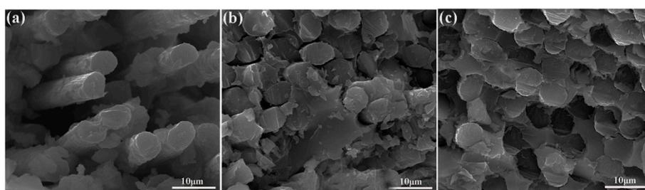
**Figure 5.** SEM morphologies of the fracture surface of MPSR composites reinforced with (a) untreated CF; (b) CF/PDA, and (c) CF/PDA/SiO<sub>2</sub>.
