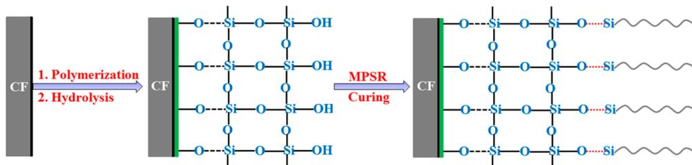
**Figure 6.** The possible mechanism of binding the SiO<sub>2</sub> layer onto the PDA pre-modified CF surface and the interfacial reaction of CF/PDA/SiO<sub>2</sub> composites.
