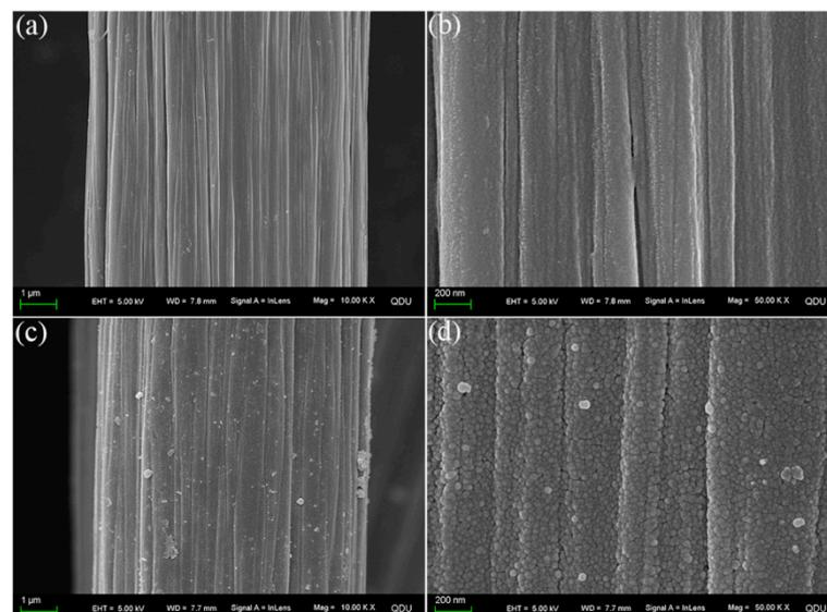
**Figure 3.** SEM images of different CFs surfaces: (a,b) CF/PDA and (c,d) CF/PDA/SiO<sub>2</sub>.
