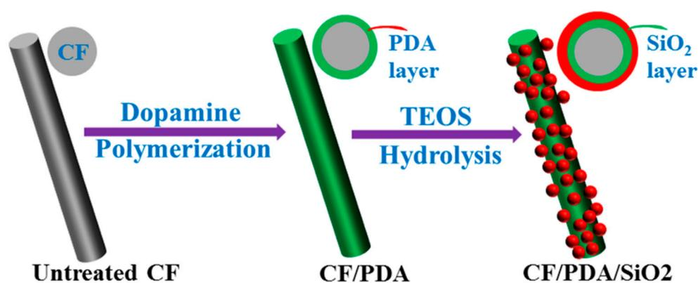
**Figure 1.** Schematic of binding SiO<sub>2</sub> coating onto the modified fiber surface via self-polymerized polydopamine.
