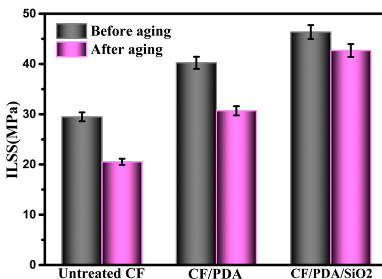
Figure 8. ILSS of composites before and after hydrothermal aging treatment.
