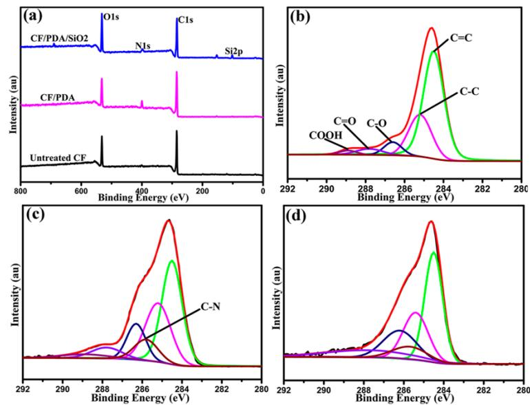
**Figure 2.** (a) Wide-scan survey XPS spectra of carbon fibers; XPS spectra of C1s peaks: (b) untreated CF, (c) CF/PDA, and (d) CF/PDA/SiO<sub>2</sub>.
