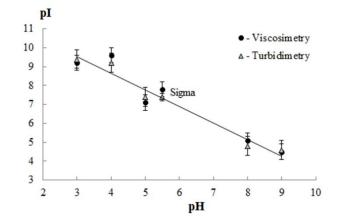
**Figure 1.** Effect of extraction pH on the isoelectric point (pI) of gelatin. Data were obtained by the methods of turbidimetry and capillary viscometry.
