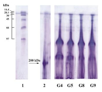
**Figure 3.** Electropherogram of gelatin samples obtained from cod skin at different pH. Electropherograms of standard low molecular weight markers (GE Healthcare) (1) and a reference sample with  $M_w = 200$  kDa (2) are shown.
