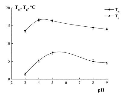
**Figure 6.** Gelling,  $T_g$ , and melting,  $T_m$ , temperatures of cod gelatin gels depending on extraction pH.  $C_G = 10$  wt.%.
