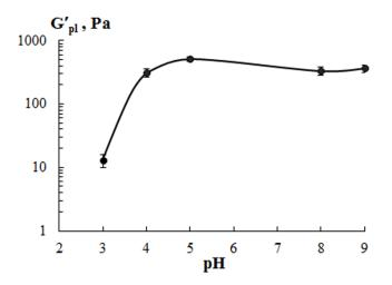
**Figure 8.** Effect of extraction conditions on the storage modulus plateau ( $G'_{pl}$ ) for cod gelatin gels.  $C_G = 10$  wt.%.
