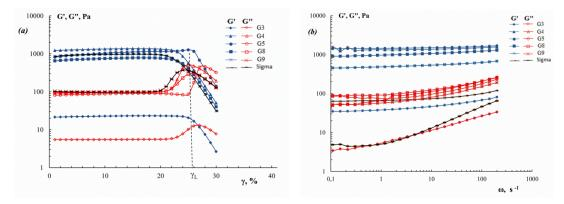
**Figure 7.** (a) Strain amplitude dependencies of the storage modulus G' (filled points) and loss modulus G'' (open points),  $\omega = 6.28 \text{ s}^{-1}$ ; (b) Frequency dependence of storage modulus G' (filled points) and loss modulus G'' (open points),  $\gamma = 2\%$ , for gels of cod gelatin extracted at different pH. C<sub>G</sub> = 10 wt.%, t = 6 °C.
