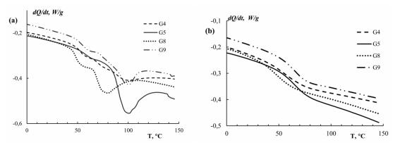
**Figure 9.** Thermograms of gelatin samples obtained at different pH (**a**) First heating cycle—determination of melting temperature and enthalpy; (**b**) second heating cycle—determination of glass transition temperature; the heating rate of 10 °C/min.
