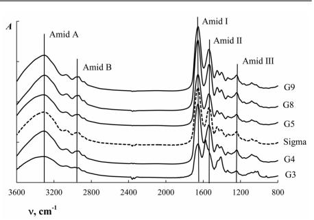
**Figure 4.** FTIR absorption spectra of cod gelatin samples obtained at different pH. pH values are given next to the appropriate spectra.
