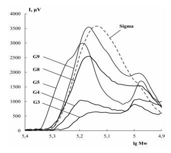
**Figure 2.** The molecular weight distribution of cod gelatin samples obtained at different pH. Extraction pH is shown as numbers with lines pointing towards curves. Chromatograms were obtained by an high-performance liquid chromatography (HPLC) method.
