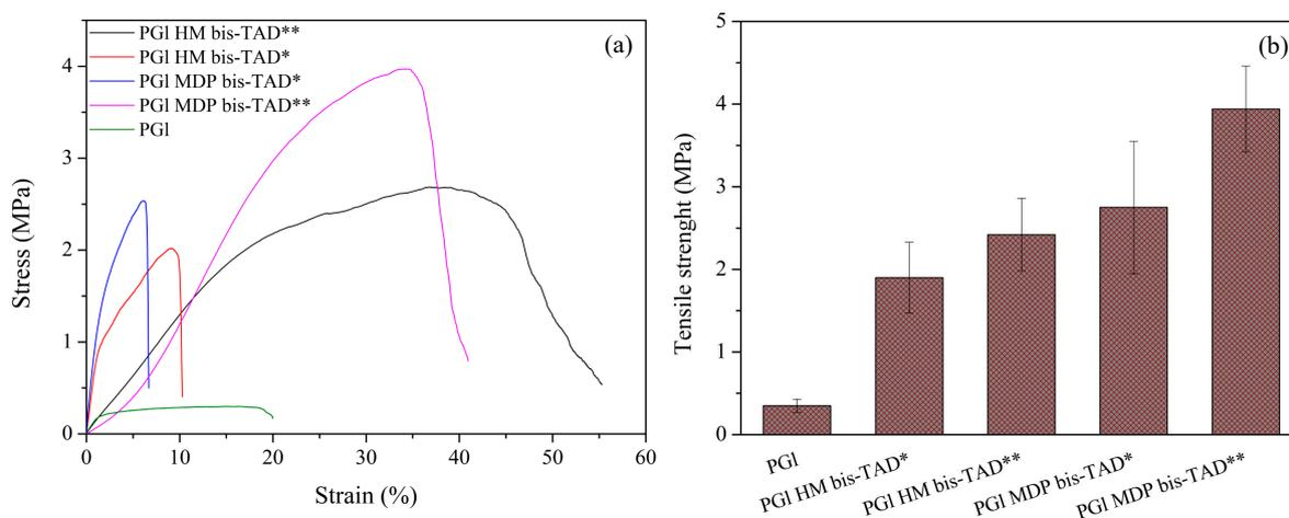
**Figure 7.** (a) Stress strain curves; (b) and tensile strength of PGI, PGI HM-bisTAD\* (first incubation), PGI HM-bisTAD\*\* (second incubation), PGI MDP-bisTAD\* (first incubation) and PGI MDP-bisTAD (second incubation) fibres.
