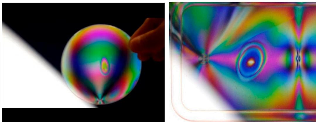
**Figure 3.** Heating to alter the color pattern observed via photo-elasticity. (Left) plastic petri dish; (right) PP box (cover). The circular/elliptical areas are produced by local heating to alter the internal stress induced by injection molding.
