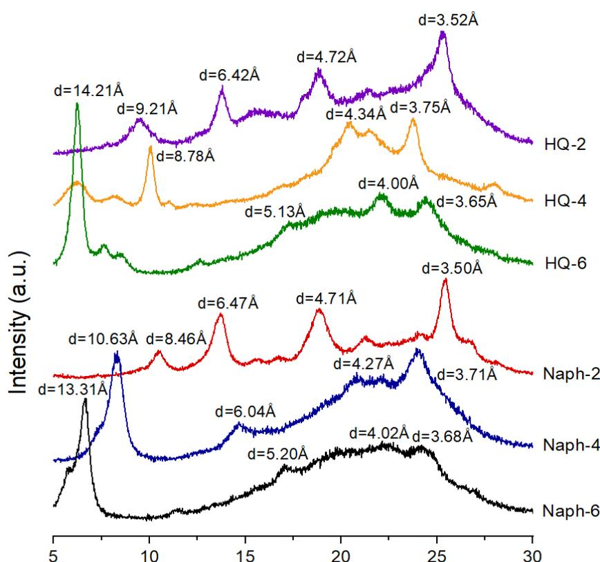
Figure 7. XRD patterns of HQ- and Naph-TLCPs.
