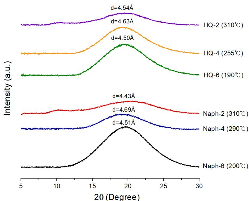
**Figure 8.** XRD patterns of HQ- and Naph-TLCPs in the LC mesogenic temperature ranges. The temperature in parentheses is the temperature at which the XRD patterns were collected.
