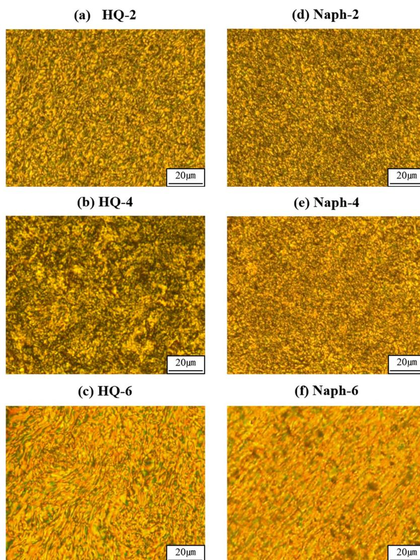
**Figure 6.** Polarized optical micrographs of (a) HQ-2 at 310 °C, (b) HQ-4 at 255 °C, (c) HQ-6 at 190 °C, (d) Naph-2 at 310 °C, (e) Naph-4 at 290 °C, and (f) Naph-6 at 200 °C (magnification 100×).
