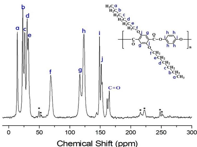
**Figure 9.** Solid state  $^{13}\text{C}$  CP/MAS NMR spectrum of HQ-6 at room temperature. The spinning sidebands are marked with asterisks.
