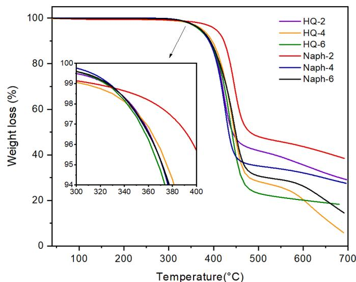
**Figure 4.** Thermogravimetric analysis (TGA) thermograms of HQ- and Naph-TLCPs.
