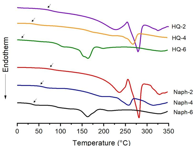
Figure 3. Differential scanning calorimetry (DSC) thermograms of HQ- and Naph-TLCPs.
