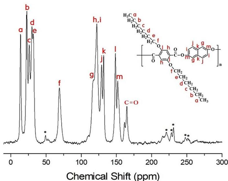
**Figure 10.** Solid state  $^{13}\text{C}$  CP/MAS NMR spectrum of Naph-6 at room temperature. The spinning sidebands are marked with asterisks.
