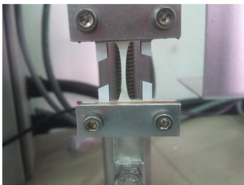
Figure 3. Set up of sample position in tensile test.
