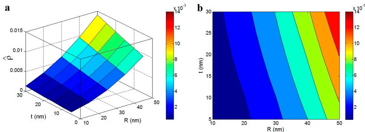
**Figure 8.** The roles of nanoparticles and interphase dimensions in the relative density of the network by “ $\phi_p$ ” predictions of Equation (7) at  $\phi_f = 0.02$ ,  $l = 5000$  nm and  $n = 100$ : (a) 3D and (b) contour plots.
