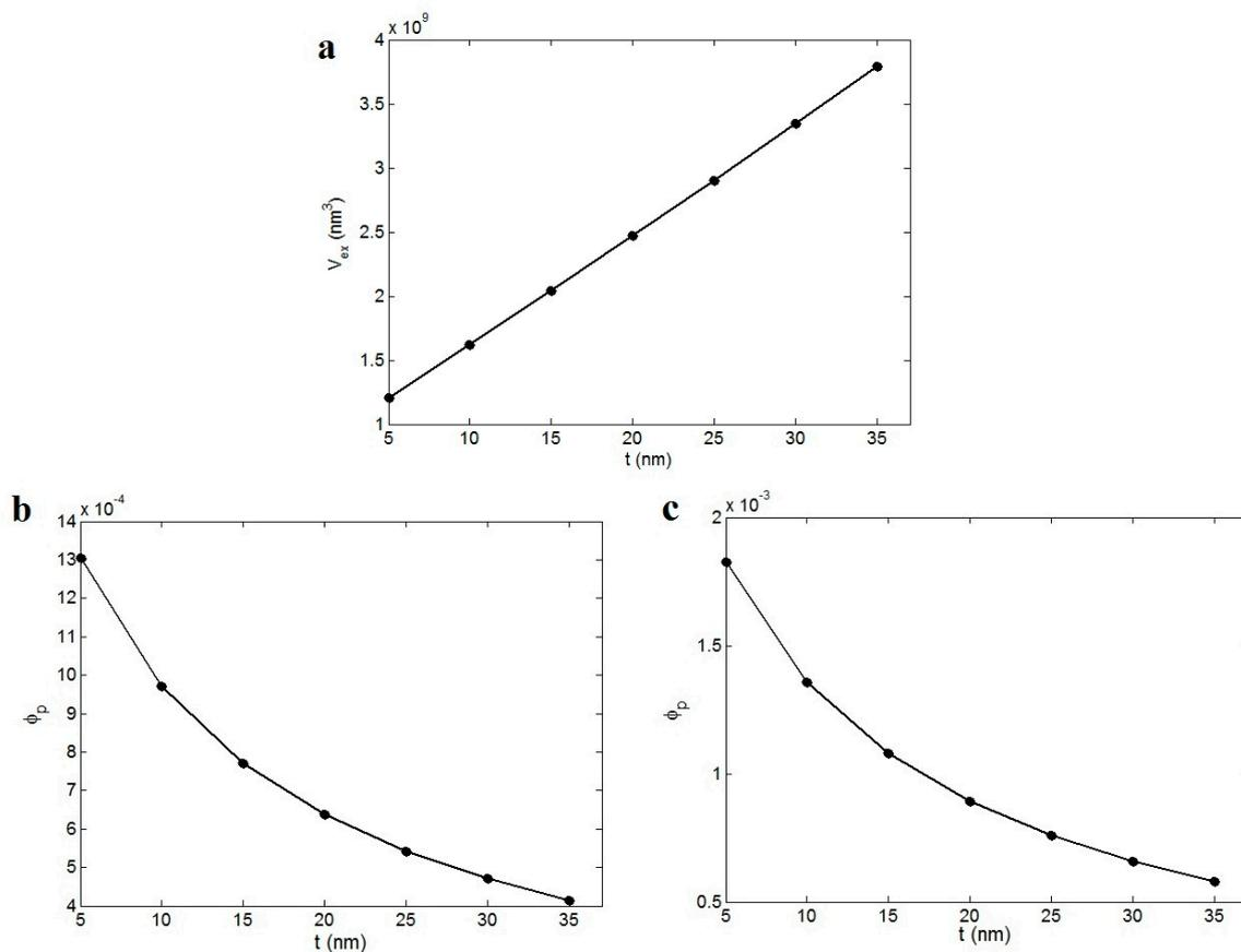
**Figure 5.** The effects of the interphase thickness on (a) excluded volume and the percolation threshold of nanoparticles according to (b) Equation (7) and (c) Equation (10) at  $R = 10$  nm and  $l = 5000$  nm.
