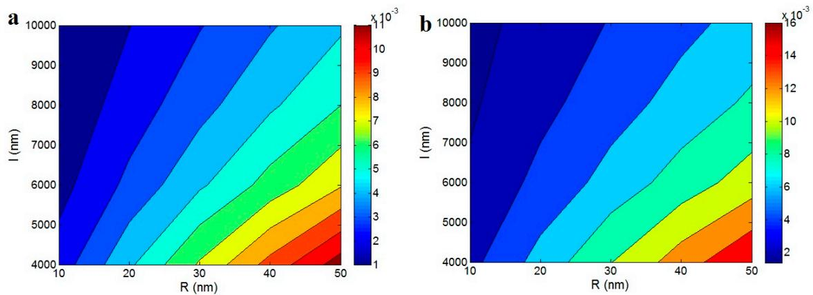
**Figure 4.** The contour plots for the influences of “R” and “l” parameters on the percolation threshold of nanoparticles based on (a) Equation (5) and (b) Equation (10).
