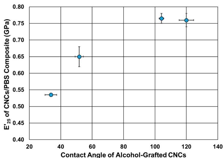
**Figure 9.** The relationship between the contact angle of the alcohol-grafted CNCs and their capabilities to reinforce PBS.
