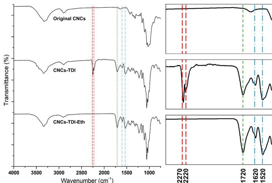
**Figure 2.** FT-IR spectra monitoring the structural changes in the CNCs upon TDI-carbamation and the following grafting of alcohols. The spectra on the right side are zoomed in a range of  $1400\text{--}2400\text{ cm}^{-1}$ .
