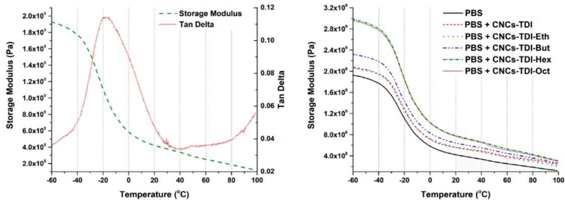
**Figure 8.** The dynamic mechanical analysis (DMA) results of the neat and reinforced PBS samples showing the glass transition temperature of PBS at around  $-17\text{ }^{\circ}\text{C}$  (Left) and the effect of the surface modification of CNCs on their reinforcement capabilities (Right).
