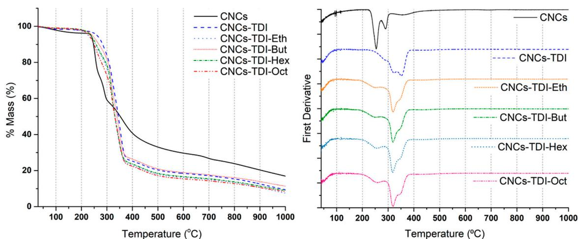
**Figure 4.** Thermogravimetric analysis (TGA) and DTG results of the CNCs before and after surface modification showing the significant change in thermal stability.
