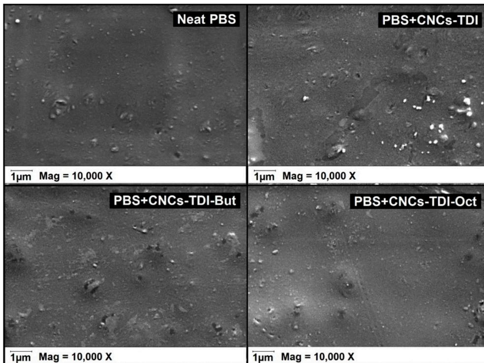
**Figure 7.** SEM images of PBS upon the addition of the modified CNCs indicating no CNC agglomeration. The small spheres were observed in all samples even the neat PBS. They are possibly a result of sample cutting.
