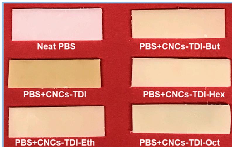
**Figure 6.** The change in the color of poly(butylene succinate) (PBS) upon processing with the modified CNCs.
