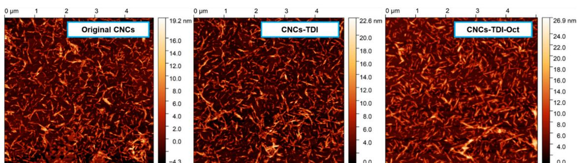
**Figure 3.** AFM height images of the CNCs before and after surface modification indicating no significant change in the morphology.
