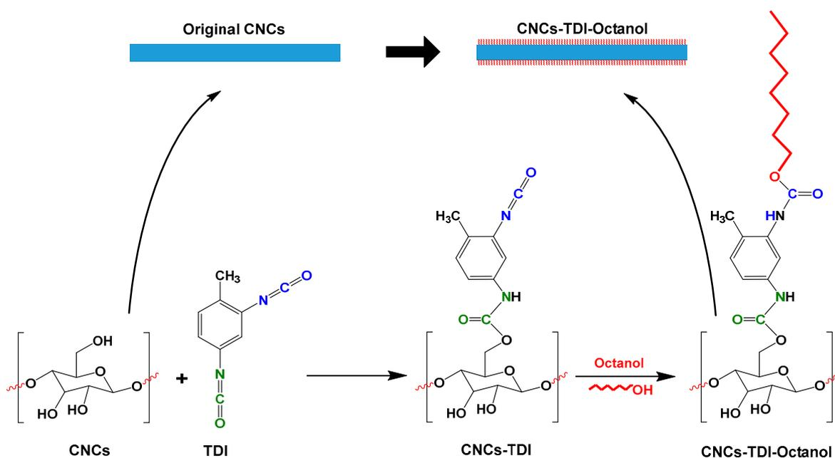
**Figure 1.** The proposed approach to tailor the hydrophilicity of cellulose nanocrystals (CNCs) by grafting alcohols of different chain lengths on the CNC surface using 2,4-toluene diisocyanate (TDI) as a linker.
