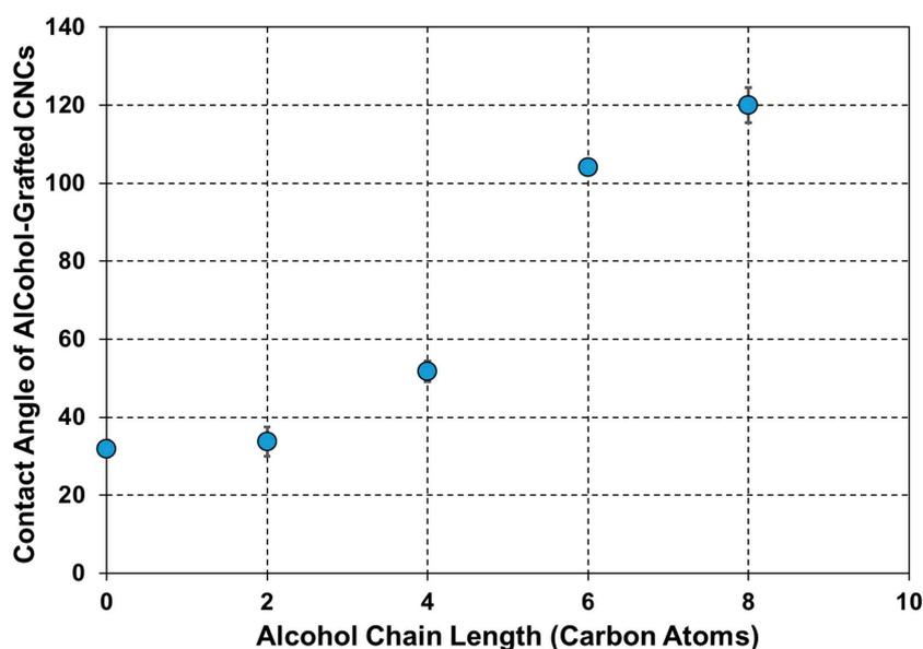
**Figure 5.** The dependence of the contact angle of the modified CNCs on the chain length of the alcohols grafted onto their surfaces.
