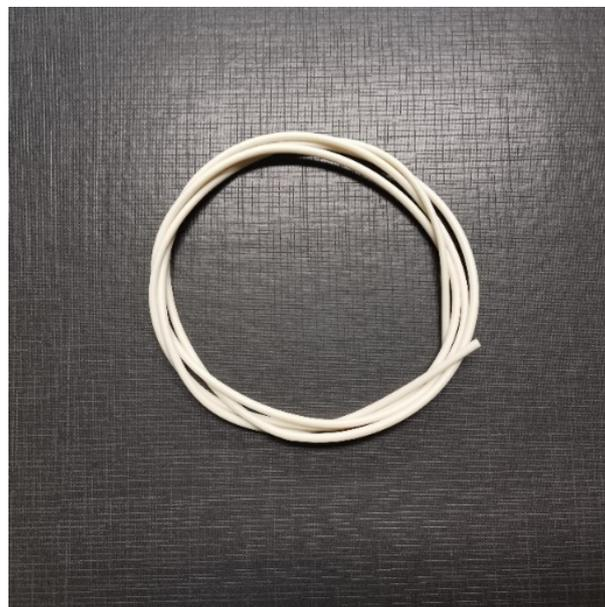
**Figure 8.** Extruded filament of ENR-50/PCL at 50/50.
