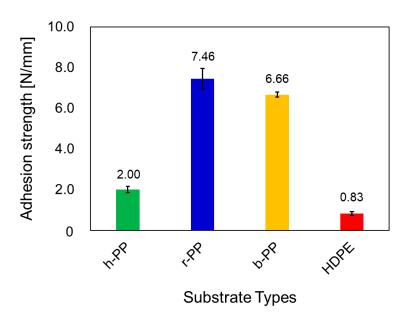
**Figure S2.** Adhesion strength of the modified h-PP attached with other substrates, which were also modified with BHA-TBAEMA under the optimized condition. These results were evaluated by the T-peel tests.
