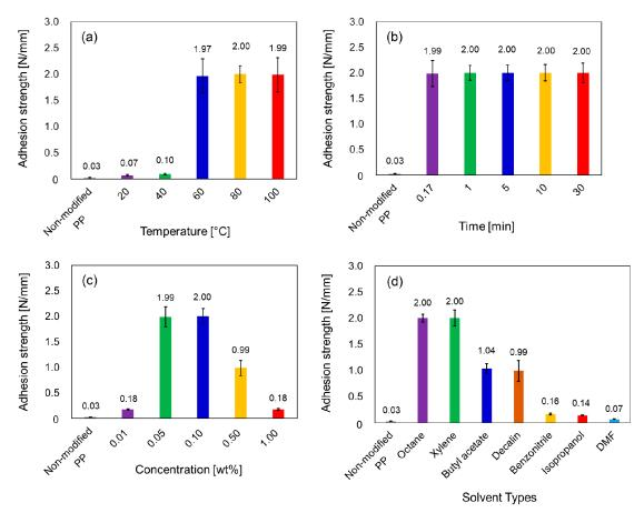
**Figure S1.** Adhesion strength of the non-modified PP and PP modified with the SCCBC evaluated by the T-peel tests: (a) 0.1 wt% of BHA-TBAEMA in xylene for 10 min at different dipping temperatures; (b) 0.1 wt% of BHA-TBAEMA in xylene at 80 °C with different dipping times; (c) BHA-TBAEMA at 80 °C for 5 min at different concentrations of BHA-TBAEMA in xylene solution; (d) 0.1 wt% of BHA-TBAEMA in different solvent types at 80 °C for 5 min.
