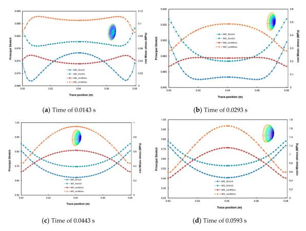
**Figure 12.** Transient evolution of the principal stretch and von Mises stresses at different instants: (a) time = 0.0143 s, (b) time = 0.0291 s, (c) time = 0.0443 s and (d) time = 0.0593 s.
