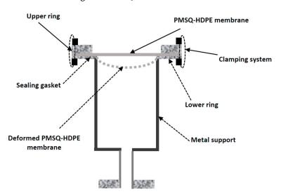
Figure 2. Fixation module.
