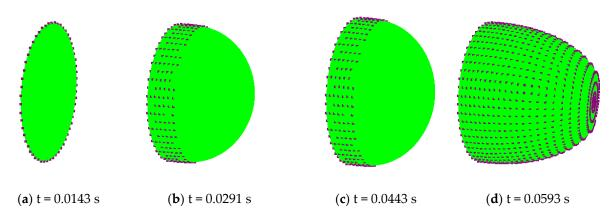
**Figure 16.** Evolution of the distribution of the contact nodes with the mold at at different instants: (a) time = 0.0143 s, (b) time = 0.0291 s, (c) time = 0.0443 s and (d) time = 0.0593 s.
