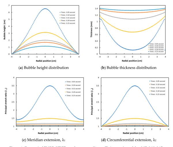
**Figure 6.** Geometrical PMSQ–HDPE membrane according to Christensen's model at 0.05, 0.10, 0.15, 0.20, and 0.25 s: (a) Bubble height, (b) Bubble thickness, (c) Stretch ration  $\lambda_1$  and (d) Stretch ration  $\lambda_2$ .
