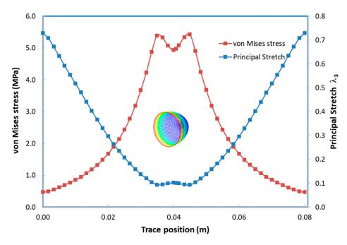
**Figure 17.** Von Mises stress and stretch ratio,  $\lambda_3$ , on the half plane of symmetry at the end of the forming cycle.
