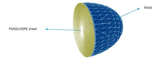
Figure 8. Geometries of the mold and the wood plastic composite (WPC) sheet.
