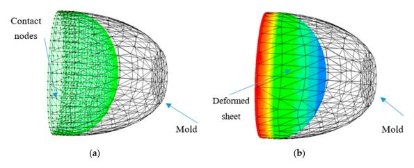
**Figure 15.** Shape of the deformed MD and principal stretch  $\lambda_3$  in the time-critical neighborhood 0.06 s. (a) Final shape of the deformed MD. (b) Distribution of the principal extensions  $\lambda_3$  in the final deformed MD.
