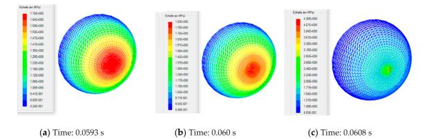
**Figure 14.** Von Mises constraints induced in the HDPE–PMSQ with the MD model in the time-critical neighborhood 0.0593 s.
