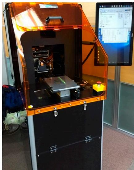
**Figure 1.** Homemade full-color material jetting (MJ) printer.
