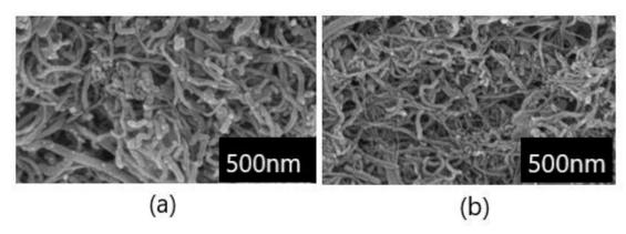
**Figure 1.** The scanning electron microscope (SEM) micrograph of carbon nanotubes network. The upper surface of entangled carbon nanotube network prepared by the filtering method from multiwalled carbon nanotubes (MWCNTs; pure) and oxidized MWCNTs (KMnO<sub>4</sub>). (a) SEM micrograph of the MWCNTs (pure). (b) SEM micrograph of MWCNTs (KMnO<sub>4</sub>).
