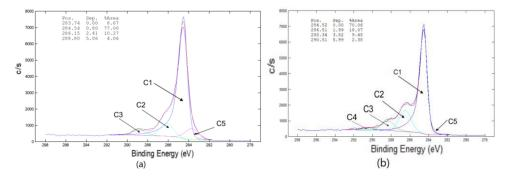
**Figure 2.** X-ray photoelectron spectroscopy (XPS) on CNT/PU and CNT/PU KMnO<sub>4</sub>. (**a**) Curve fitting of the C 1s carbon spectrum of the MWCNTs (pure). (**b**) Curve fitting of the C 1s carbon spectrum of MWCNTs (KMnO<sub>4</sub>).
