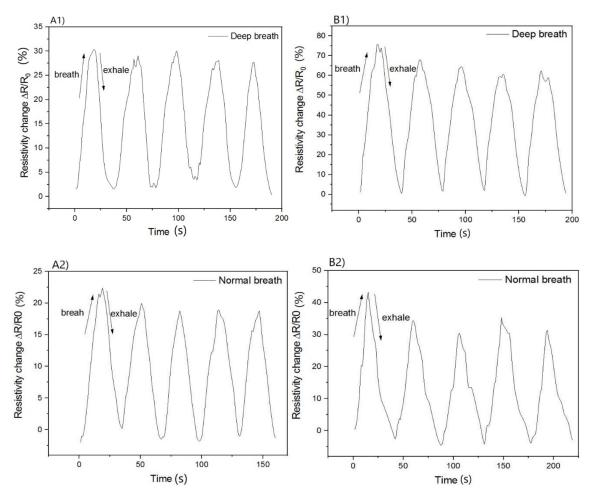
**Figure 8.** Response to a change in relative resistance,  $\Delta R/R_0$ , of carbon nanotube sensors (MWCNTs/KMnO<sub>4</sub>) integrated into the T-shirt to monitor human breath. The comparison of deep breath and normal breath for both volunteers (A1,A2,B1,B2).
