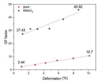
**Figure 6.** Dependence of gauge factor (GF) with increasing deformation for MWCNTs (pure) and oxidized MWCNTs (KMnO<sub>4</sub>) sensors.
