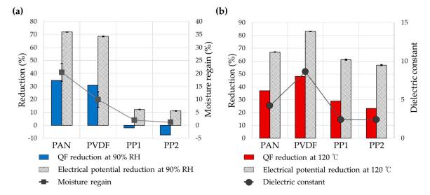
**Figure 6.** Effect of humidity and temperature on the electric potential and quality factor (QF). (a) Material's moisture regain vs. the reduction of QF and electric potential with humidity aging; (b) material's dielectric constant vs. the reduction of QF and electric potential with thermal aging.
