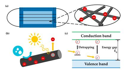
**Figure 1.** Scheme of study concept. (a) Electret fibers applied to a filtering respirator; (b) charge decay with the exposure to moisture and heat; (c) charge detrapping phenomenon.
