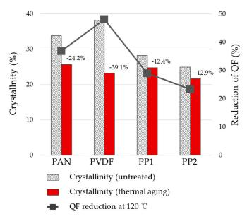
**Figure 7.** Relationship of crystallinity reduction (%) and QF reduction (%) with thermal aging. The percentage values above the bar charts are the reduction % of crystallinity with thermal aging.
