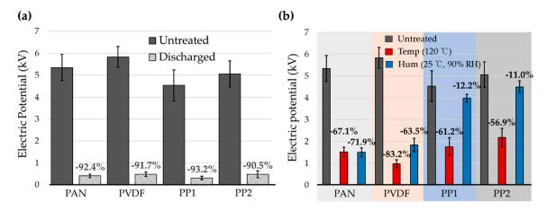
**Figure 3.** Electric potential measured for electret filters under various conditions. (a) Comparison of electric field from electret filter and discharged filter; (b) electric potential of electret filters before and after aging. Numerical values above the bar chart are the reduction (%) of electric potential for treatments, compared to the untreated filters.
