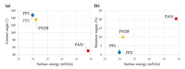
**Figure 2.** Materials' affinity to water. (a) Contact angle and surface energy; (b) moisture regain and surface energy.
