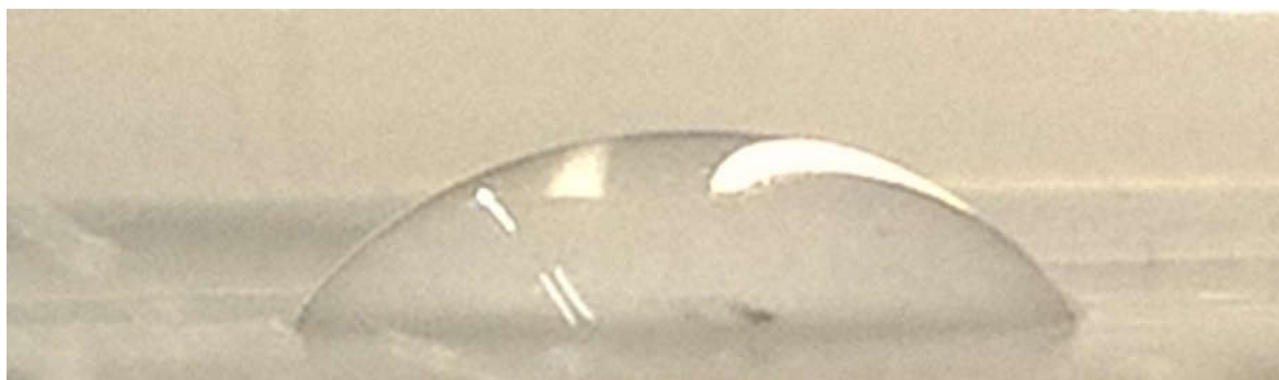
Figure S6. The image of a drop of water on the surface of a polymer film.
