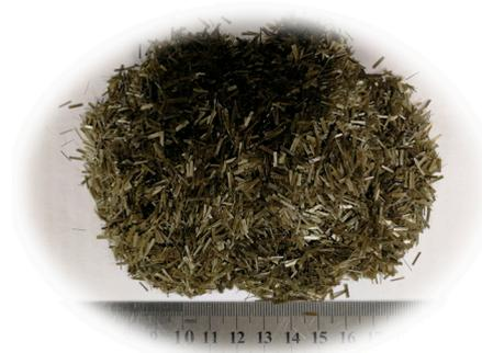
**Figure 1.** Basalt fiber with length of 6 mm used in this study.
