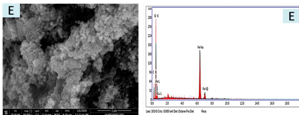
**Figure 3.** SEM and EDX of (A) Cellulose, (B) Acell), (C) nNiO/Acell, (D) nCuO/Acell and (E) nFe<sub>3</sub>O<sub>4</sub>/Acell nanocomposites.
