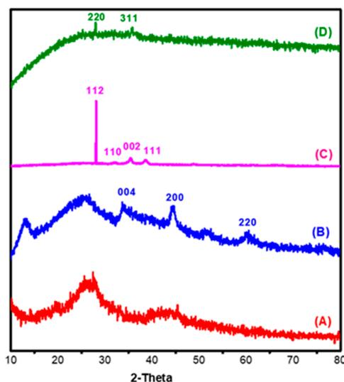
**Figure 2.** XRD pattern for (A) Acell, (B) nNiO/Acell, (C) nCuO/Acell and (D) nFe<sub>3</sub>O<sub>4</sub>/Acell nanocomposite.
