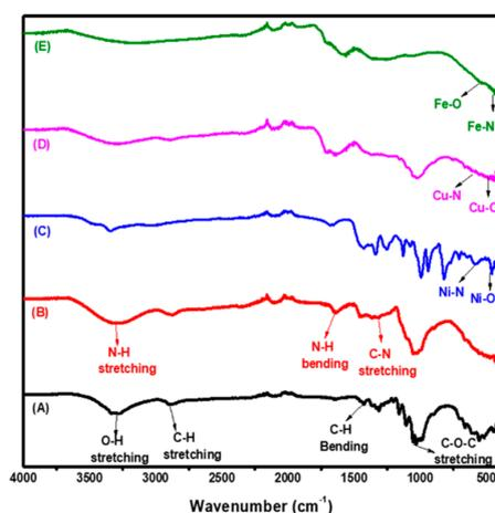
**Figure 1.** Fourier transform-infrared spectroscopy (FT-IR) spectra for (A) Cellulose, (B) aminated cellulose (Acell), (C) nNiO/Acell, (D) nCuO/Acell and (E) nFe<sub>3</sub>O<sub>4</sub>/Acell nanocomposite.
