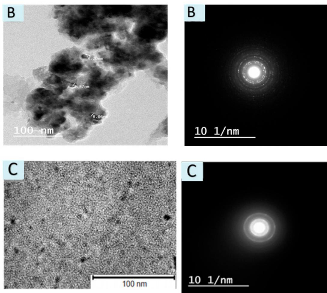
**Figure 4.** Transmission electron microscopy (TEM) and selected area electron diffraction (SAED) pattern for (A) nNiO/Acell, (B) nCuO/PAC and (C) nFe<sub>3</sub>O<sub>4</sub>/Acell nanocomposites.
